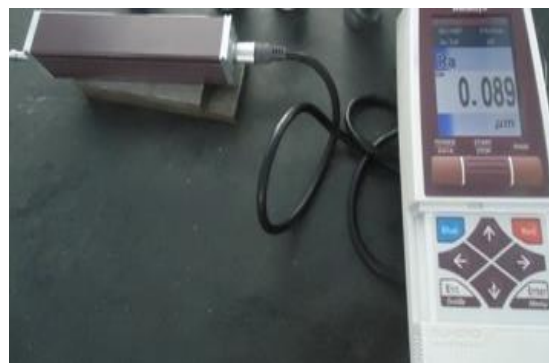
Fig. 4. Surface roughness measurement tester.
