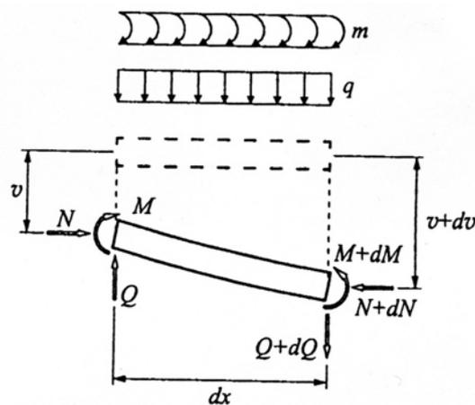
Fig. 1. Elementary unit of a beam considered.
