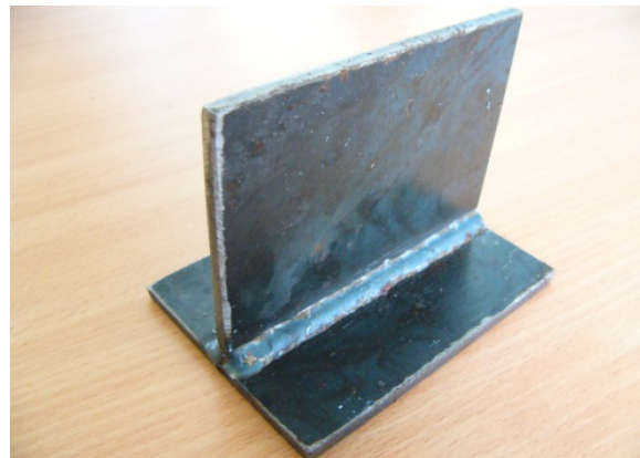
Fig. 1. View of S 235 welded T-joint.
