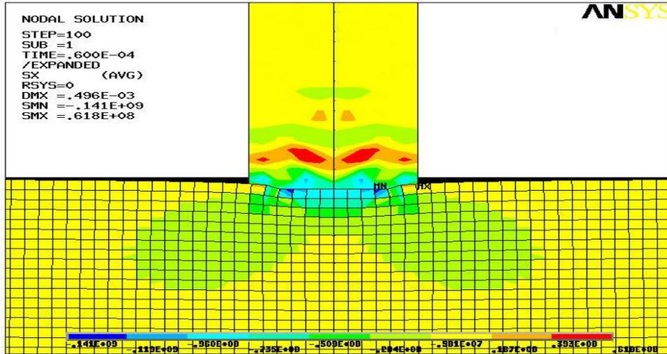
Fig. 3. Typical field of the horizontal stresses in the process interaction of a stud with asphalt media.
