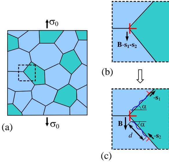
**Fig. 6.** Geometry of the dislocation reaction in a deformed nanocrystalline nanocomposite containing metallic and ceramic nanograins. (a) Nanocrystalline nanocomposite under a tensile load (general two-dimensional view). (b,c) A dislocation with the Burgers vector  $\mathbf{B}-\mathbf{s}_1-\mathbf{s}_2$  (b) transforms into the dislocations with the Burgers vectors  $\mathbf{B}$ ,  $-\mathbf{s}_1$  and  $-\mathbf{s}_2$  (c).
