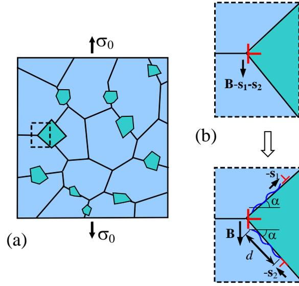
**Fig. 7.** Geometry of the dislocation reaction in a deformed microcrystalline-metal-matrix nanocomposite containing ceramic nanoparticles at grain boundaries. (a) Microcrystalline-metal-matrix nanocomposite under a tensile load (general two-dimensional view). (b,c) A dislocation with the Burgers vector  $\mathbf{B}-\mathbf{s}_1-\mathbf{s}_2$  (b) transforms into the dislocation with the Burgers vectors  $\mathbf{B}$ ,  $-\mathbf{s}_1$  and  $-\mathbf{s}_2$  (c).
