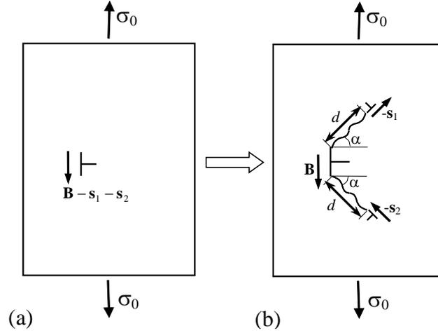
**Fig. 3.** Geometry of the dislocation reaction in a deformed crystalline solid. A dislocation with the Burgers vector  $\mathbf{B} - \mathbf{s}_1 - \mathbf{s}_2$  (a) transforms into the dislocation with the Burgers vector  $\mathbf{B}$  joined by generalized stacking faults with the dislocations with the Burgers vector  $-\mathbf{s}_1$  and  $-\mathbf{s}_2$  (b).
