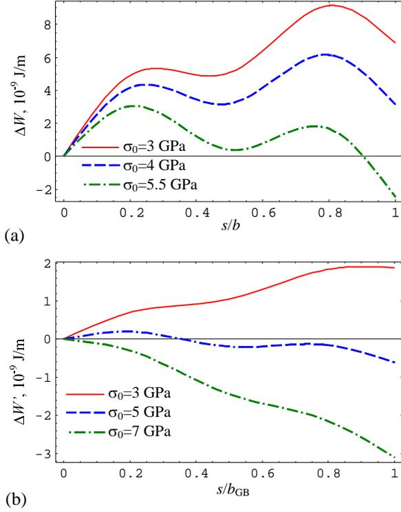
**Fig. 4.** The energy variations  $\Delta W$  (a) and  $\Delta W'$  (b) associated with the emission of lattice (a) and grain boundary (b) dislocations by ideal local shears vs. the normalized magnitudes  $s/b$  (a) and  $s/b_{GB}$  (b) of the dislocation Burgers vectors.
