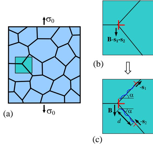
**Fig. 5.** Geometry of the dislocation reaction in a deformed nanocrystalline solid. (a) Nanocrystalline solid under a tensile load (general two-dimensional view). (b,c) A dislocation with the Burgers vector  $\mathbf{B}-\mathbf{s}_1-\mathbf{s}_2$  (b) transforms into the dislocation with the Burgers vector  $\mathbf{B}$  joined by grain boundary generalized stacking faults with the dislocations with the Burgers vector  $-\mathbf{s}_1$  and  $-\mathbf{s}_2$  (c).
