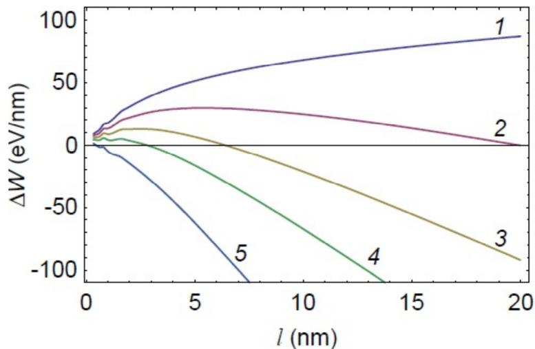
**Fig. 2.** (Colour online) Typical dependences of the total energy change  $\Delta W$  on the distance  $l$  moved by the partial dislocations in copper. The dependences are calculated, for  $b_{gb}=1 \text{ \AA}$ ,  $\varphi=15^\circ$ , and  $\tau=0.001 \text{ G}$ ,  $0.02 \text{ G}$ ,  $0.04 \text{ G}$ ,  $0.06 \text{ G}$ , and  $0.1 \text{ G}$  (curves 1, 2, 3, 4, and 5, respectively).
