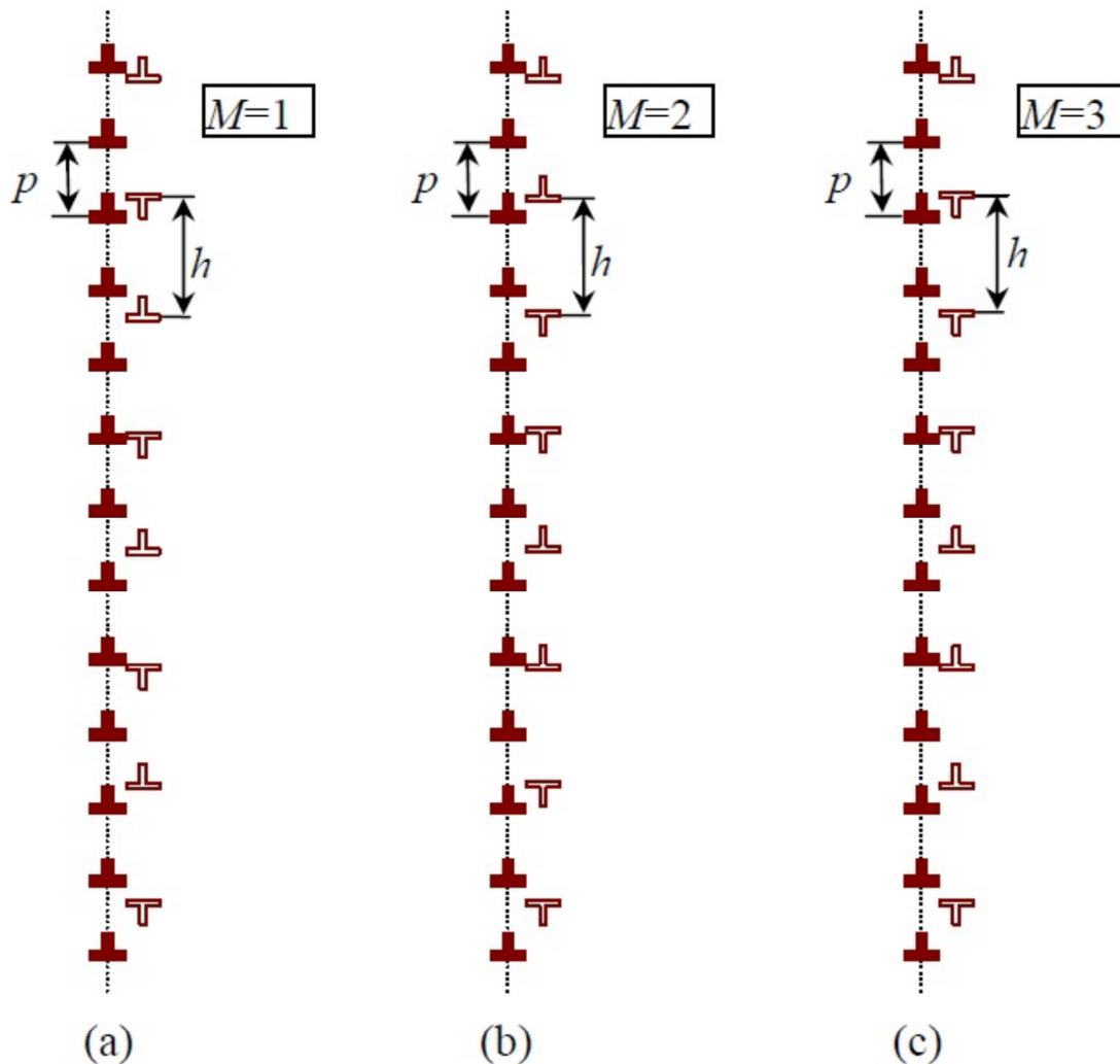
**Fig. 3.** (Color online) Dislocation structures of deformation-distorted grain boundaries for various values of parameter  $M$  (for details, see text). (a)  $M = 1$ ; (b)  $M = 2$ ; (c)  $M = 3$ .
