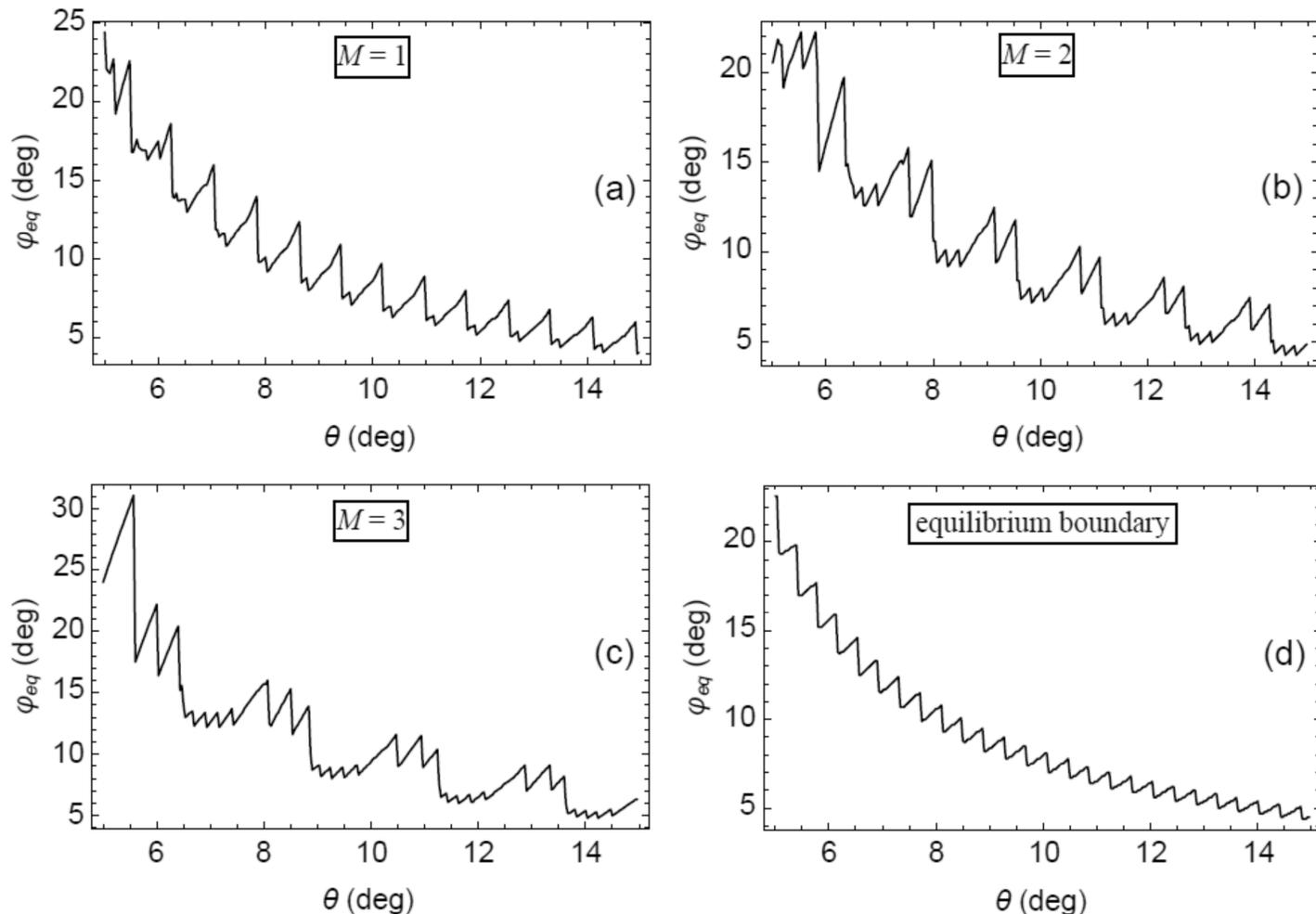
**Fig. 6.** Dependences of equilibrium rotation angle  $\varphi_{eq}$  on tilt misorientation angle  $\theta$ , for deformation-distorted grain boundaries specified by (a)  $M = 1$ ; (b)  $M = 2$ ; and (c)  $M = 3$ ; as well as for (d) non-distorted grain boundary (free from non-equilibrium dislocations). Other parameters of the system are taken as:  $\tau = 0.05D$ ,  $\alpha = 45^\circ$ ,  $p = h$ , and  $d = 100b$ .
