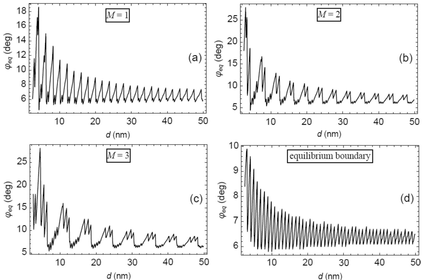
**Fig. 7.** Dependences of equilibrium rotation angle  $\varphi_{eq}$  on the parameter  $d$  (close to the length of the rotating grain boundary), for deformation-distorted grain boundaries specified by (a)  $M = 1$ ; (b)  $M = 2$ ; and (c)  $M = 3$ ; as well as for (d) non-distorted grain boundary (free from non-equilibrium dislocations). Other parameters of the system are taken as:  $\tau = 0.05D$ ,  $\alpha = 45^\circ$ ,  $h = 5b$ , and  $p = h$ .
