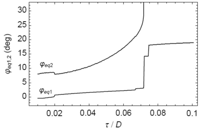
**Fig. 9.** Dependences of equilibrium rotation angles  $\varphi_{\text{eq1}}$  and  $\varphi_{\text{eq2}}$  on the applied shear stress  $\tau$ , for deformation-distorted split grain boundary specified by the following values of parameters:  $M = 1$ ,  $\alpha = 45^\circ$ ,  $h = 5b$  ( $\theta \approx 11^\circ$ ),  $p = h$ , and  $d = 100b$ .
