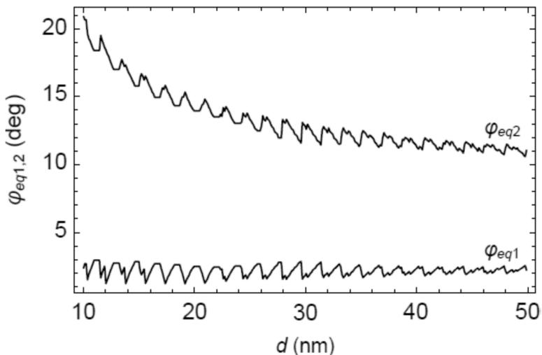
**Fig. 11.** Dependences of equilibrium rotation angles  $\varphi_{eq1}$  and  $\varphi_{eq2}$  on the parameter  $d$  (close to the length of the initial grain boundary AB), for deformation-distorted split grain boundary specified by the following values of parameters:  $M = 1$ ,  $\alpha = 45^\circ$ ,  $h = 5b$  ( $\theta \approx 11^\circ$ ),  $\rho = h$ , and  $\tau = 0.05D$ .
