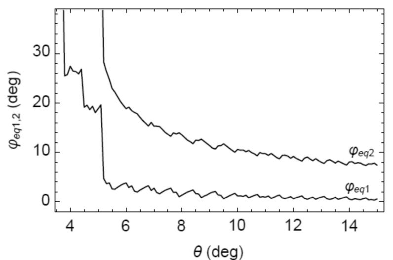
**Fig. 10.** Dependences of equilibrium rotation angles  $\varphi_{\text{eq1}}$  and  $\varphi_{\text{eq2}}$  on tilt misorientation  $\theta$ , for deformation-distorted split grain boundary specified by the following values of parameters:  $M = 1$ ,  $\alpha = 45^\circ$ ,  $p = h$ ,  $d = 100b$ , and  $\tau = 0.03D$ .
