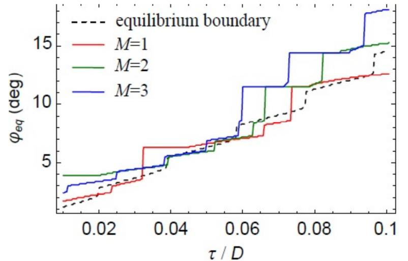
**Fig. 5.** (Color online) Dependences of equilibrium rotation angle  $\varphi_{\text{eq}}$  on the applied shear stress  $\tau$ , for deformation-distorted grain boundaries specified by  $M = 1, 2$ , and 3 as well as for the following values of other parameters:  $\alpha = 45^\circ$ ,  $h = 5b$  ( $\theta \approx 11^\circ$ ),  $p = h$ , and  $d = 100b$ . Dependence  $\varphi_{\text{eq}}(\tau)$  for non-distorted grain boundary (free from non-equilibrium dislocations) is shown as dashed curve.
