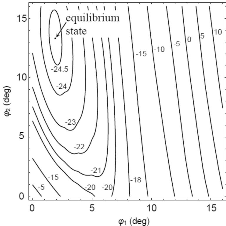
**Fig. 8.** Map of the energy change  $\Delta W_{\text{split}}(\varphi_1, \varphi_2)$ , for deformation-distorted split grain boundary specified by  $M = 1$  and for the following values of other parameters:  $\tau = 0.05D$ ,  $\alpha = 45^\circ$ ,  $h = 5b$  ( $\theta \approx 11^\circ$ ),  $p = h$ , and  $d = 100b$ . The energy change is given in units of  $Db^2$ .
