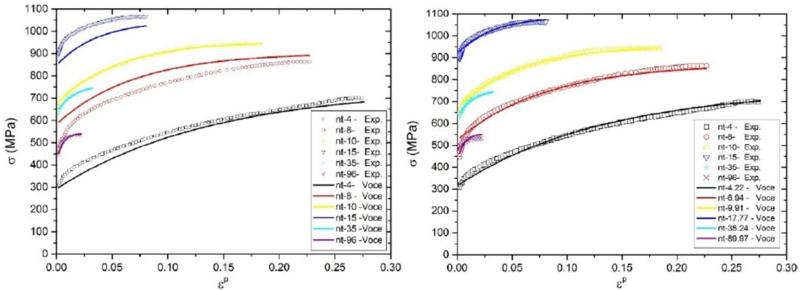
**Fig. 4.** The fit of the various size-dependent true stress-strain curves for nt-Cu specimens with varying twin thickness. The modified size-dependent Voce model employed was based on Eqs. (11) and (12) with the unique set of the parameter values used for all curves given in Table 2: (a) twin thickness is the same as that reported in [12]. (b) slightly modified twin thickness.
