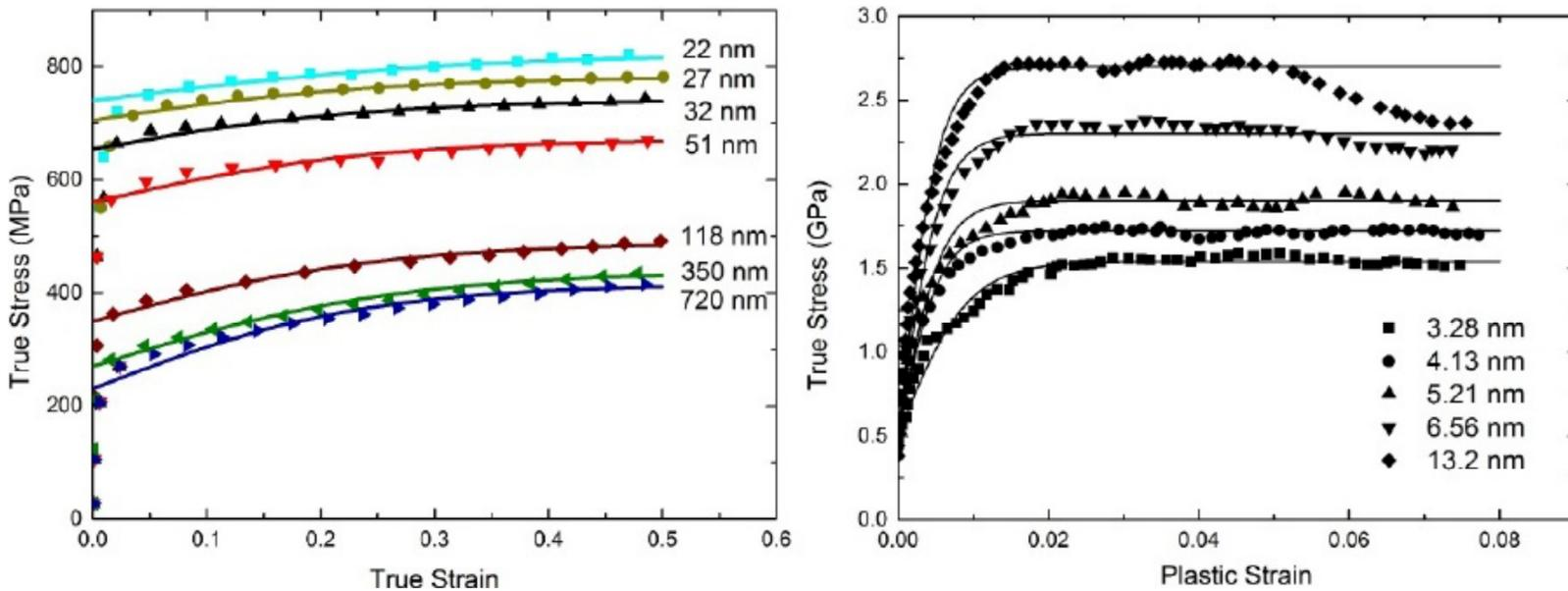
**Fig. 1.** (a) Fitting the grain size dependence of nanocrystalline copper (nc-Cu) specimens showing a HP type of “hardening” behavior. (b) Comparison between model predictions and simulations for nc-Cu sample of showing a IHP type of “hardening” behavior.
