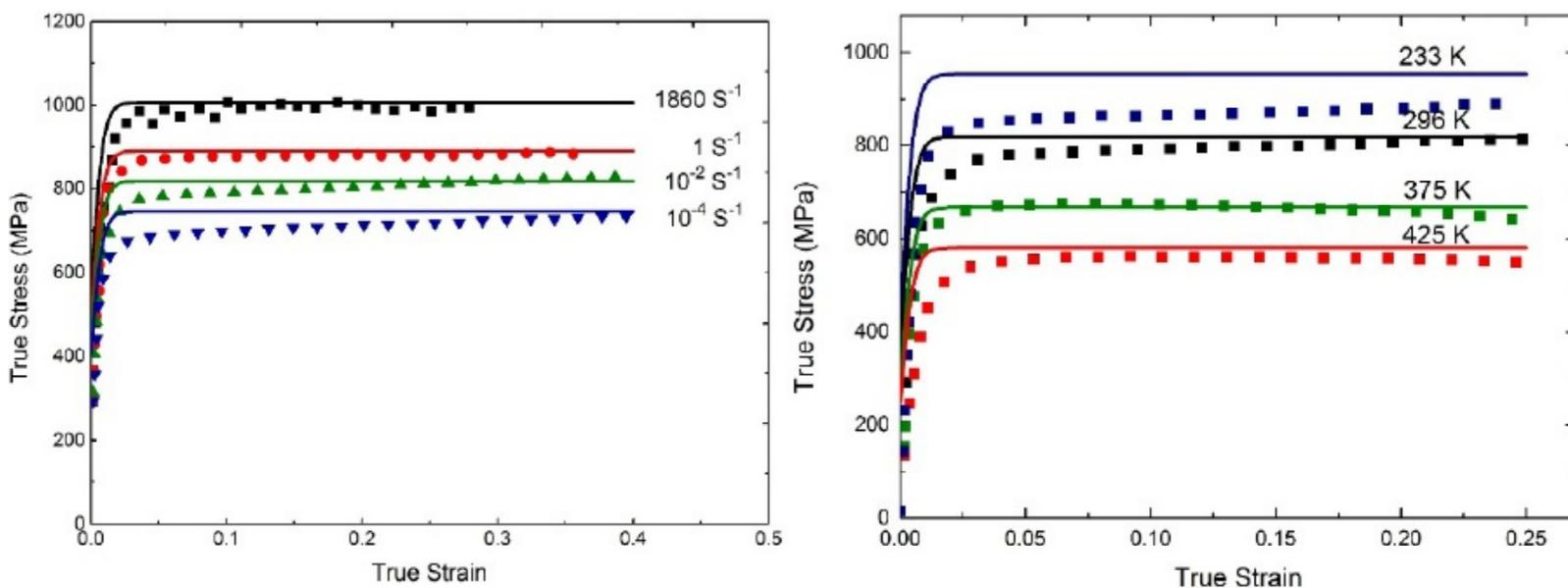
**Fig. 2.** (a) Fitting the strain rate dependence of nanocrystalline copper (nc-Cu) specimens. (b) Fitting the temperature dependence of nanocrystalline copper (nc-Cu) specimens.
