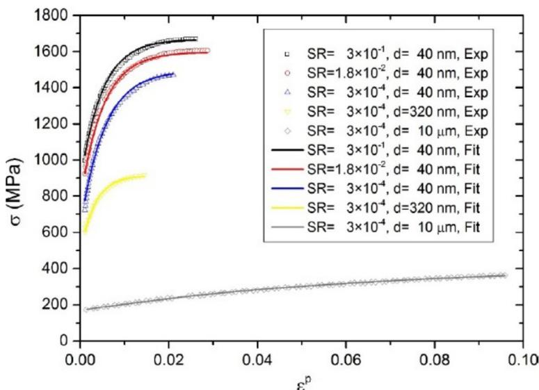
**Fig. 3.** Fitting the simultaneous effect of grain size and strain rate dependence on the stress-strain response of nc-Ni.
