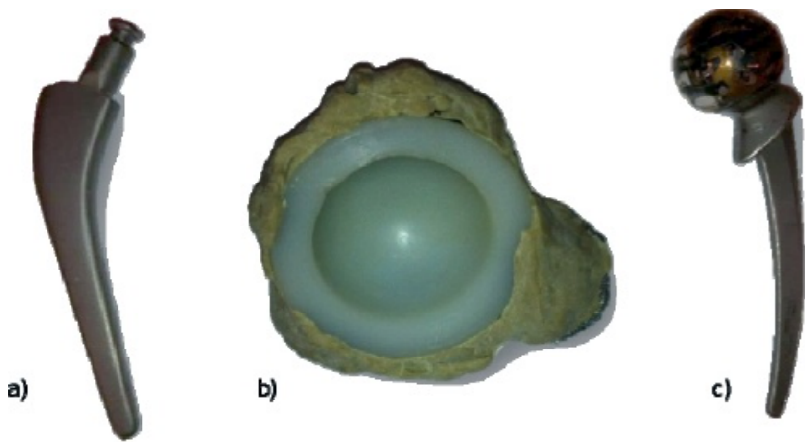
Fig. 1. Hip prosthesis components: a) the stem femoral of titanium, b) the acetabular component of polyethylene with the cement and c) the stem and head femoral of titanium.
