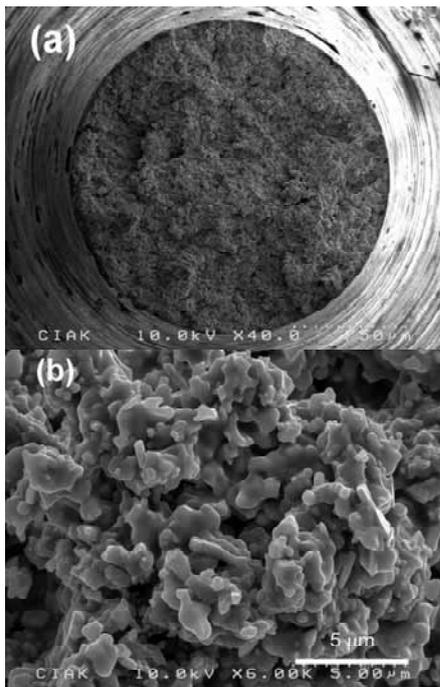
**Fig. 5.** Fracture surface of VN-1 alloy (under 150  $\mu\text{m}$ ) tested at 500  $^{\circ}\text{C}$  at the strain rate of  $10^{-2} \text{ s}^{-1}$ . (a) fracture surface, (b) magnified picture of the fracture surface.
