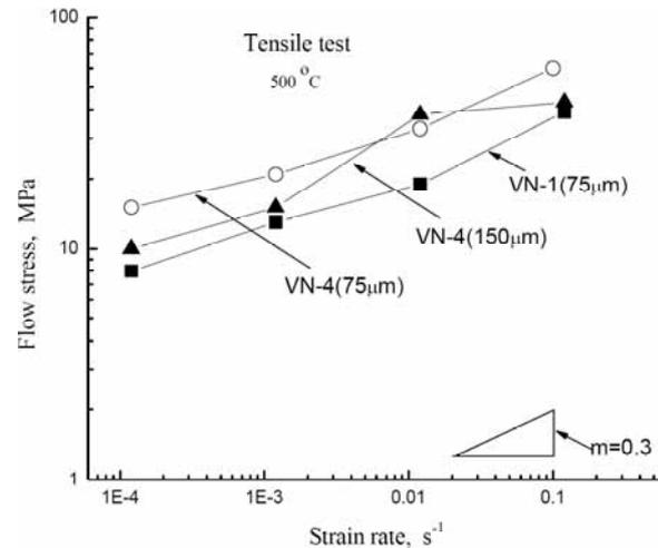
**Fig. 6.** Relationship between flow stress and strain rate of VN-1 and VN-4 alloys.
