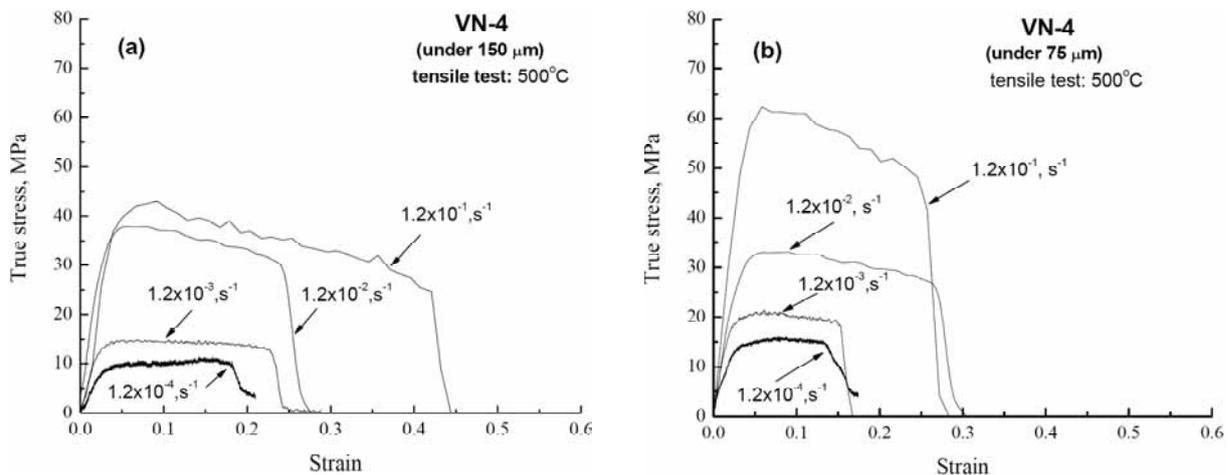
**Fig. 3.** Change of stress-strain curves of VN-4 alloy by strain rate. (a) for powders under  $150\ \mu\text{m}$  in size, (b) for powder under  $75\ \mu\text{m}$ .
