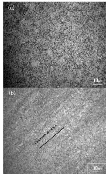
**Fig. 1.** Microstructures of the extruded VN-4 (75 μm) alloy, (a) perpendicular and (b) parallel to the extrusion direction.
