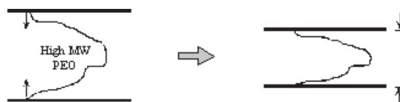
Fig. 7. Schematic illustration of bridging flocculation occurs in polymer nanocomposite in the presence of high molecular weight polymer.
