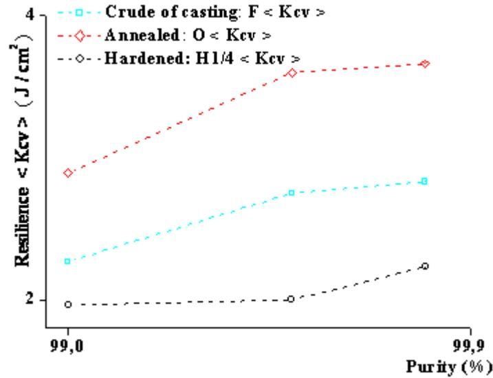
Figure 5: Group of graphs (average resilience Kcv – purity degree) of comparison in averaging a series of five identical specimens of the aluminum commercial of the three states: crude of casting noted: F, annealing noted: O and hardened noted: H1/4.
