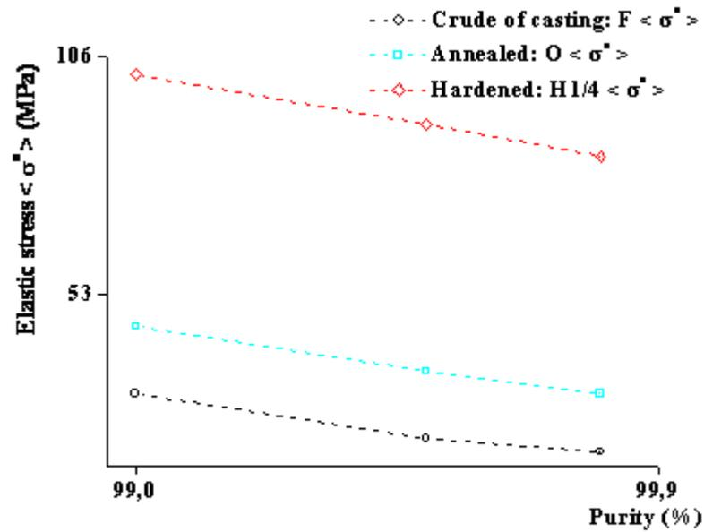
Figure 1: Group of graphs (average stress of elasticity – purity degree) of comparison in averaging a series of five identical specimens of the aluminum commercial of the three states: crude of casting noted: F, annealing noted: O and hardened noted: *H1/4*.
