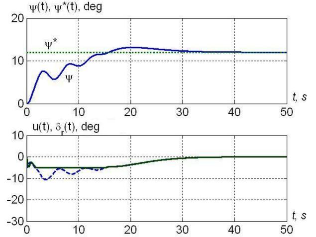
Fig. 8. Step responses in the aircraft control system in the case of reference signal  $\psi^* = 12^\circ$ ; the time histories of PID-controller output signal  $u_r(t)$  (solid line) and the rudder deflection angle  $\delta_r(t)$  (dashed line). Control law (10), (15),  $k_A = 2$ .
