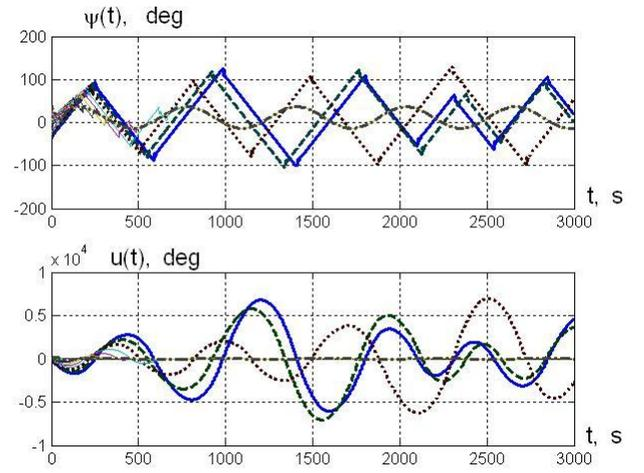
Fig. 5. A set of the time histories  $\psi(t)$ ,  $u_r(t)$  in the case of control law (8), (10) for reference signal  $\psi^*(t) = \psi_0^* + \psi_{\max}^* \sin(\Omega t)$  and various initial conditions  $\psi(0)$ .
