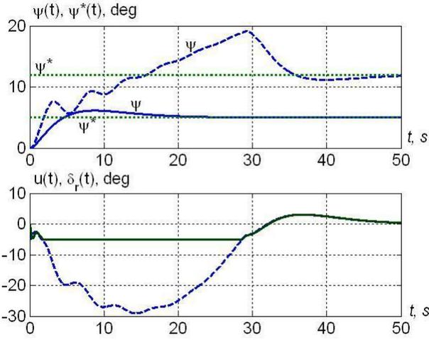
Fig. 3. Step responses in the aircraft control system in the case of reference signal  $\psi^* = 5^\circ$  (solid line) and  $\psi^* = 12^\circ$  (dashed line); the time histories of PID-controller output signal  $u_r(t)$  (solid line) and the rudder deflection angle  $\delta_r(t)$  (dashed line) in the case of reference signal  $\psi^* = 12^\circ$ .
