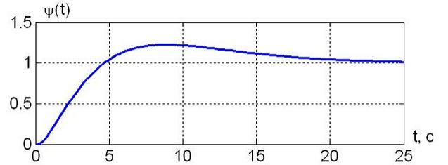
Fig. 2. Step response in the “nominal” closed-loop aircraft control system. Control law (8),  $\sigma_r(t) \equiv u_r(t)$ .
