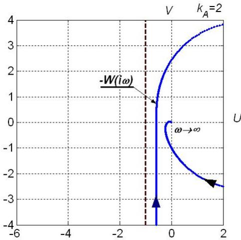
Fig. 7. Nyquist chart for the aircraft control system with AW-correction. Control law (10), (15),  $k_A = 2$ .
