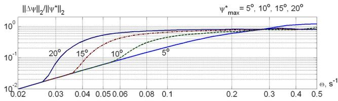
Fig. 11. Sensitivity function  $\mathbb{S}(\psi_{\max}^*, \omega) = \|\Delta\psi\|_2 / \|\psi^*\|_2$ . Control law (10), (15) ( $k_A = 2$ ) as  $\psi_{\max}^* = 5^\circ \div 25^\circ$ .
