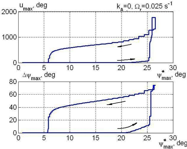
Fig. 4. Plots of the control signal magnitude  $u_r$  and the reference error  $\Delta\psi(t)$  versus the reference signal magnitude in the case of control law (8), (10).
