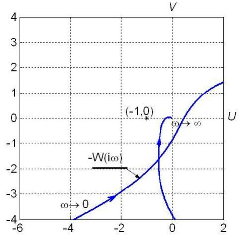
Fig. 1. Nyquist chart for the open-loop aircraft control system. Control law (8).
