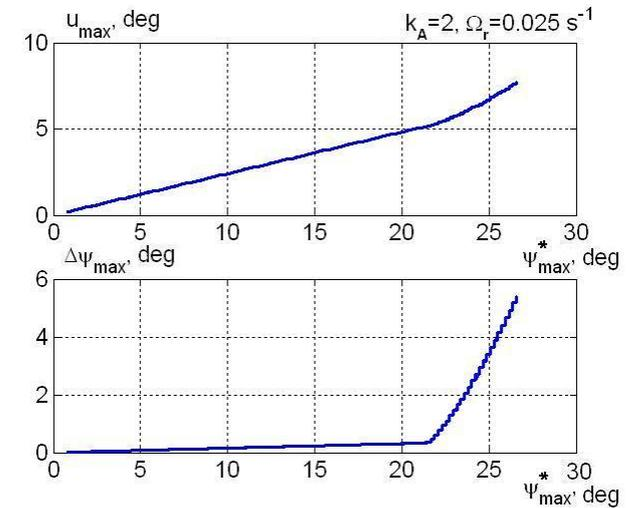
Fig. 9. Plots of the control signal magnitude  $u_r$  and the reference error  $\Delta\psi(t)$  versus the reference signal magnitude. Control law (10), (15),  $k_A = 2$ .
