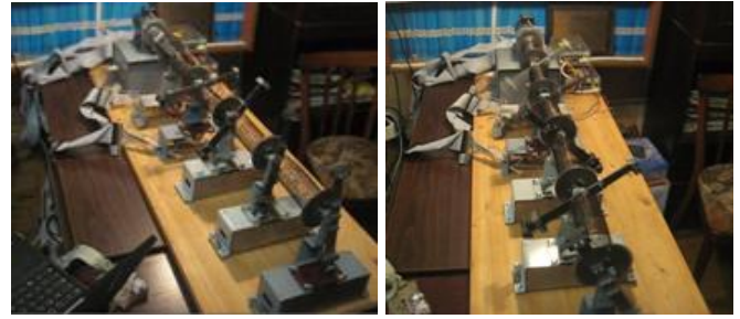
Fig. 6. Inphase ( \omega = 6 \text{ s}^{-1} ) and antiphase ( \omega = 9 \text{ s}^{-1} ) synchronization of pendulums.
