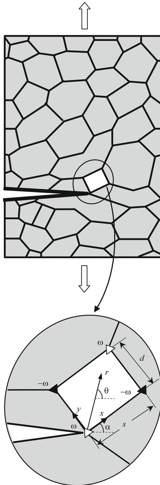
**Fig. 2.** Special rotational deformation in a deformed nanocrystalline specimen containing a mode I crack: (a) general view and (b) the magnified inset highlights a disclination quadrupole near the crack tip.
