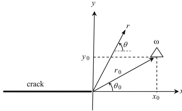
Fig. A1. Wedge disclination in a medium with a semi-infinite crack.
