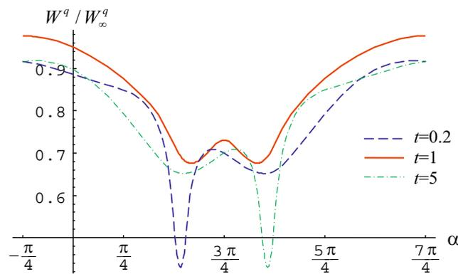
**Fig. A3.** Ratio  $W^q/W_\infty^q$  of the energy  $W^q$  of a disclination quadrupole near a crack tip to the energy  $W_\infty^q$  of a similar quadrupole in an infinite uncracked solid, as a function of the angle  $\alpha$ , for various values of the quadrupole aspect ratio  $t$ .
