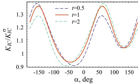
**Fig. 3.** Dependences of the normalized fracture toughness  $K_{IC}/K_{IC}^\sigma$  on the angle  $\alpha$ , characterizing the orientation of the deformed grain near the crack tip, for various values of the ratio  $t$  of the sizes of grain facets.
