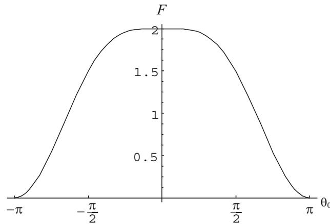
**Fig. A2.** Function  $F(\theta_0)$  characterizing the dependence of the energy of a wedge disclination in a solid with a semi-infinite crack (in units of  $D\omega^2r_0^2/2$ ) on the angular disclination coordinate  $\theta_0$ .
