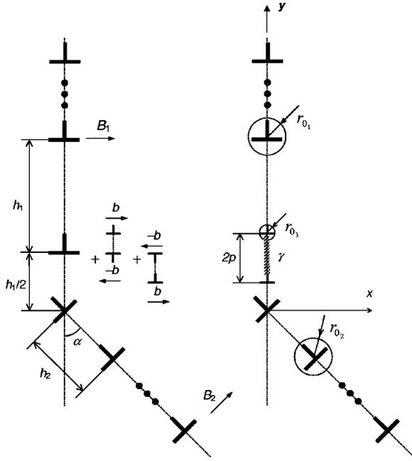
FIG. 2. Low-angle boundary structure 1-2. (a) Two facets of a low-angle boundary consisting of perfect dislocations with one dislocation being replaced by a split dislocation configuration at facet junction. (b) Split dislocation configuration is represented as a perfect dislocation and two dipoles of partial dislocations.
