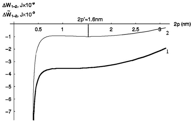
FIG. 3. Dependences of the characteristic energy differences ( $\Delta W_{1-2}$  and  $\Delta \tilde{W}_{1-2}$ ) on interspacing  $2p$  between partial dislocations forming a split dislocation configuration at facet junction (solid curve 1) and central part of a boundary facet (curve 2).
