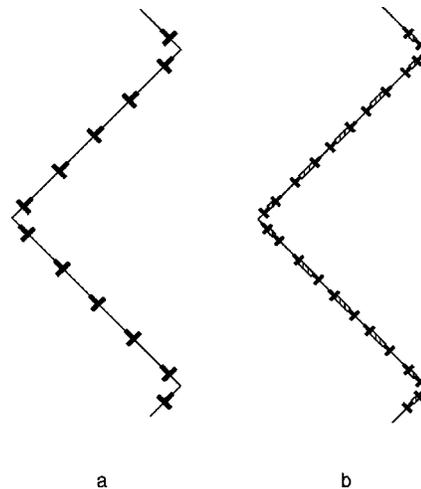
FIG. 1. Structures of faceted tilt boundaries in high- $T_c$  superconductors: (a) conventional and (b) split structures.
