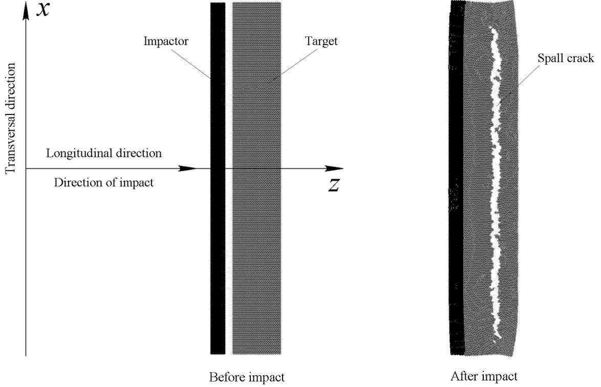
Figure 1: The computation model of the impact loading.
