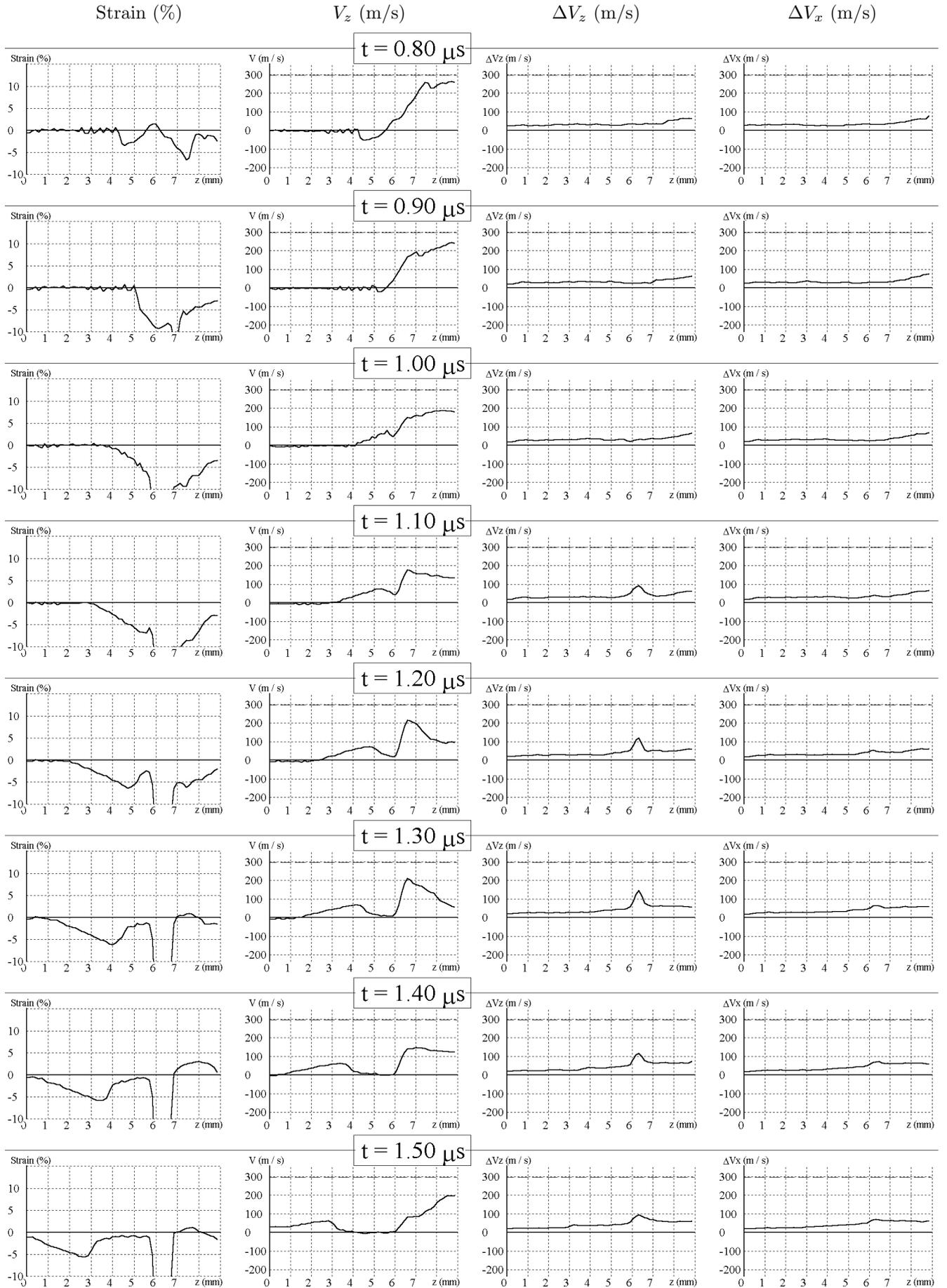
Figure 6: Spall formation in the target ( $0.9 \mu s < t < 1.6 \mu s$ ).
