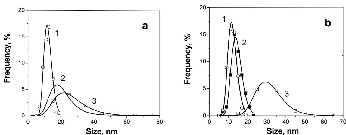
**Fig. 1.** Size distributions of particles prepared by CVC process using argon as a carrier gas: (a) as-prepared iron particles: decomposition temperature is 400 °C (curve 1), 750 °C (curve 2), and 1100 °C (curve 3); (b) sample 1 heated to 300 °C (curve 1), 400 °C (curve 2), and 700 °C (curve 3).
