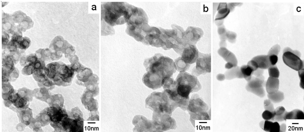
**Fig. 4.** TEM images of particles: heating to (a) 400 °C, (b) 500 °C, (c) 700 °C at a rate of 10 K/min.
