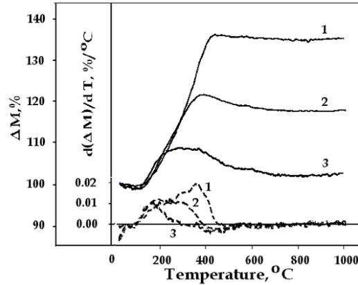
**Fig. 5.** Relative mass ( $\Delta M$ ) (solid lines) and  $d(\Delta M)/dT$  (dashed lines) of iron nanoparticles versus heating temperature ( $T$ ) upon heating at a rate of 10K/min. Mean particles size is (1) 25 nm, (2) 19.6 nm and (3) 11.8 nm.
