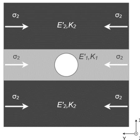
**Fig. 1.** The structure of the fracture between layers with different stress values
