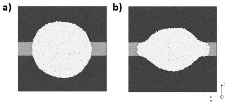
**Fig. 2.** Examples of the steady-state hydraulic fracture model in the fractured layer obtained by particle dynamics method. Black dots denote side layers. Grey dots denote the productive layer. White dots denote the fracture zone: a) the initial fracture; b) the fracture growing process
