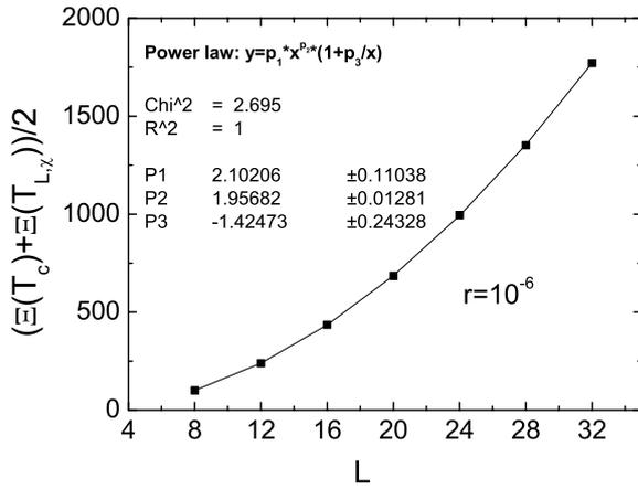
**Fig. 3.** Scaling behavior of dominant magnetic subspaces (CrMMS). The average of the two temperatures (critical and susceptibility's pseudocritical temperature) of the scaled extensions are fitted to the power law shown.
