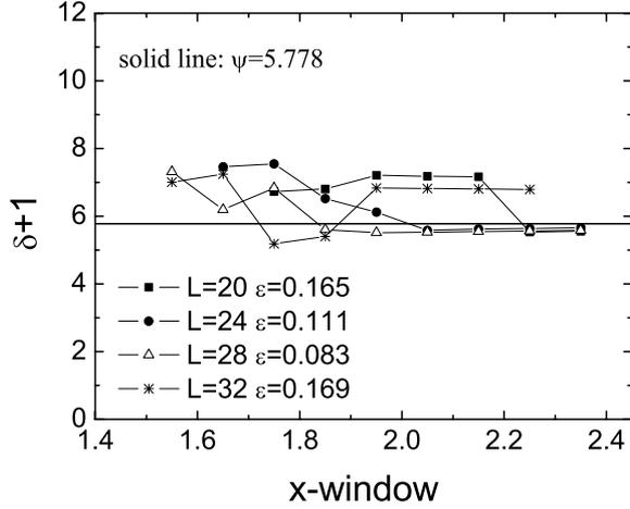
**Fig. 6.** An attempt to observe the value of the critical exponent  $\delta+1$  by fitting our data to Eq. (14). Note that, in these fits we have used  $x$ -windows corresponding to 100 magnetization values and we have suppressed the prefactor term by setting  $\psi=1$ . The solid line shows the literature's estimate of  $\delta+1$ .
