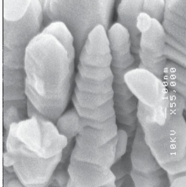
**Fig. 2.** (a) Stacking ABCABCABC in FCC crystal, with large circles on A layer, small circles on B layer, and small open circles on C layer; (b) Scanning electron microscopy image of Cu  $\langle 111 \rangle$  nanorods.
