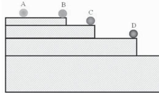
**Fig. 3.** Schematic of adatom diffusion on flat surface and down steps.
