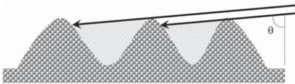
Fig. 1: Schematic of geometrical shadowing.
