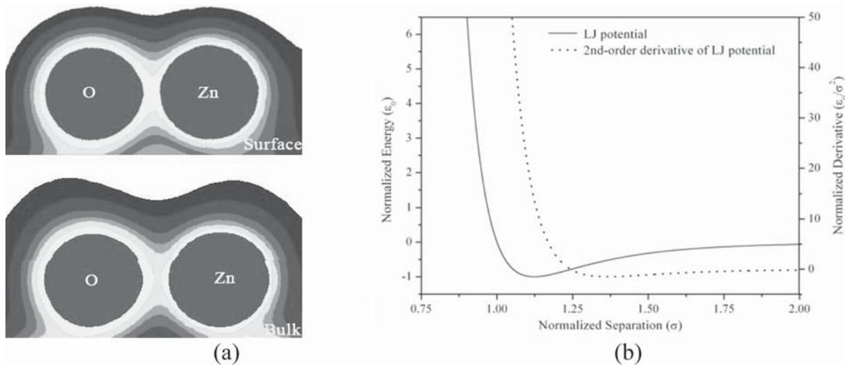
**Fig. 5.** (a) Electron density distribution along a bulk bond and a surface bond in ZnO; (b) energy and curvature as a function of atomic separation according to Lennard-Jones (LJ) potential.
