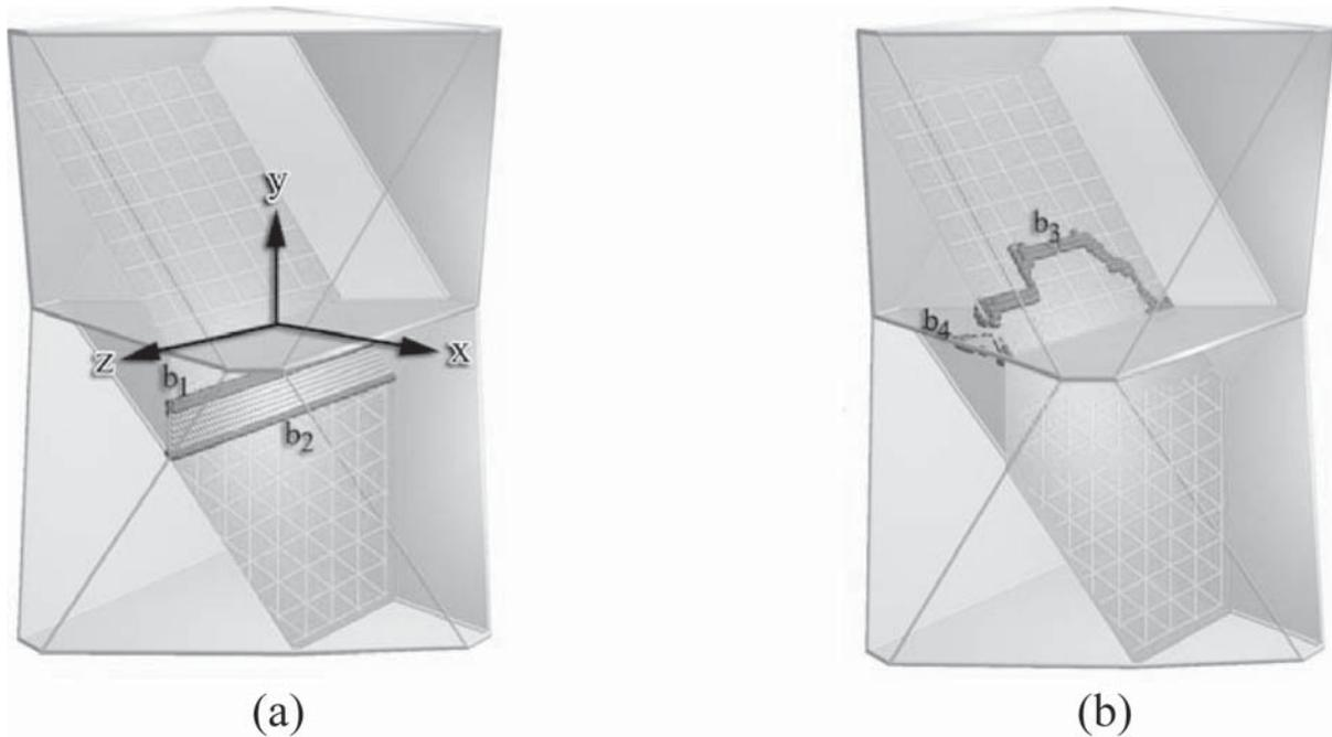
**Fig. 6.** A complete dislocation consisting of two Shockley partial dislocations on Cu{111} glide plane (a), and a complete dislocation on Cu{100} after penetrating a twin boundary (b).
