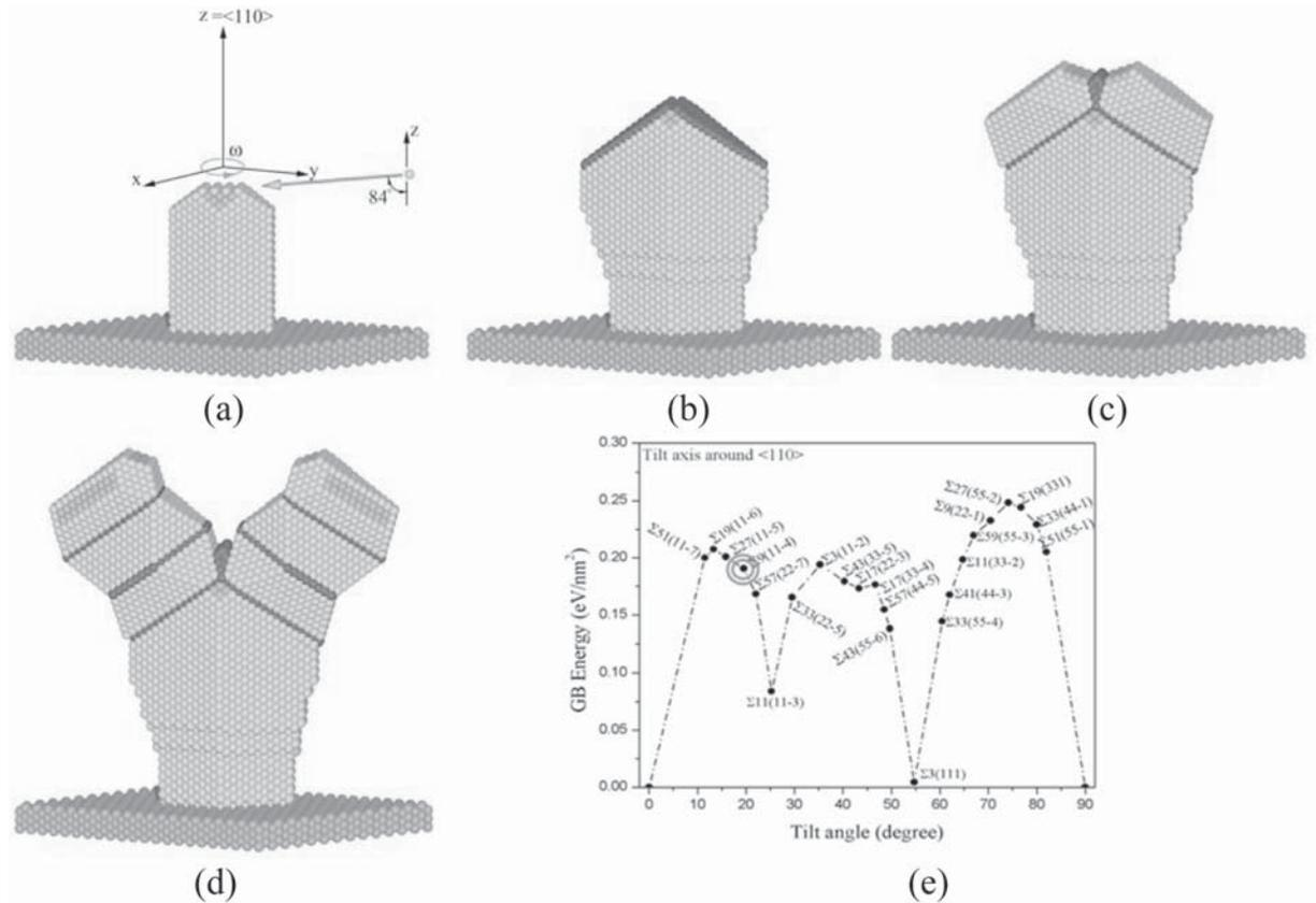
**Fig. 4.** Conceptual design of nanorods branching (a-d), and grain boundary (GB) formation energy showing high energy GBs vs low energy  $\Sigma 3$  twin GB.
