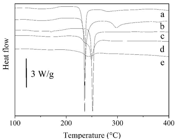
**Fig. 3.** DSC traces of: (a) Mg60 alloy, cone slices of 4 mm diameter; (b) Mg60 alloy, as quenched ribbon; (c) Mg51 alloy, as quenched ribbon; (d) Mg51 alloy, cone slices of 1 mm diameter; (e) Mg51 alloy, cone slices of 4 mm diameter. The heating rate was 40 °C/min.
