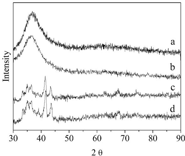
**Fig. 1.** XRD patterns of: (a) Mg51 as quenched ribbon; (b) Mg60 cone slices of 4 mm diameter; (c) Mg51 cone slices of 2 mm diameter; (d) Mg51 cone slices of 4 mm diameter.
