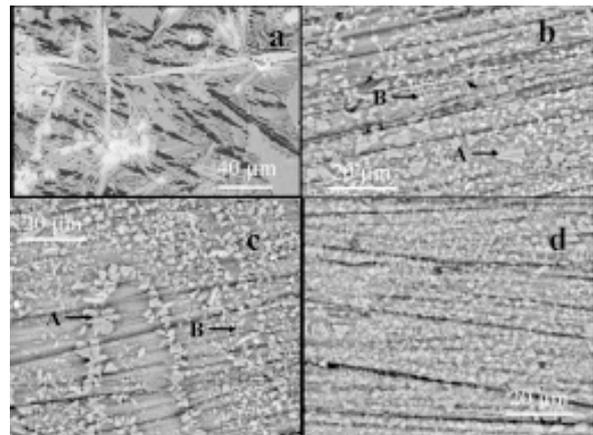
**Fig. 2.** SEM image (backscattered electrons) of Mg51 alloy: (a) master alloy; (b) cone slices of 4 mm diameter; (c) cone slices of 3 mm diameter; (d) cone slices of 2 mm diameter.
