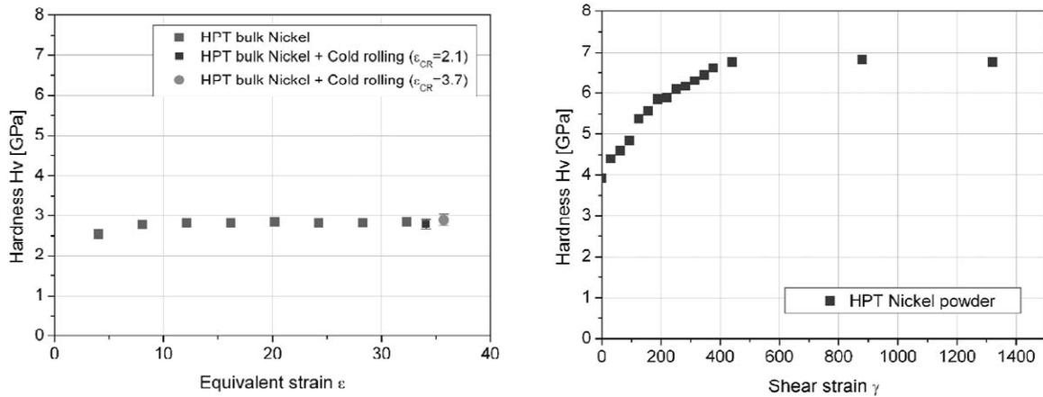
**Fig. 6.** (a) Microhardness of bulk HPT deformed Ni at room temperature as a function of the applied equivalent shear strain. The microhardness values of the Ni samples which were additionally cold rolled to two different strains are also shown. (b) Microhardness of HPT consolidated oxidized Ni powder sample as a function of the applied equivalent shear strain.
