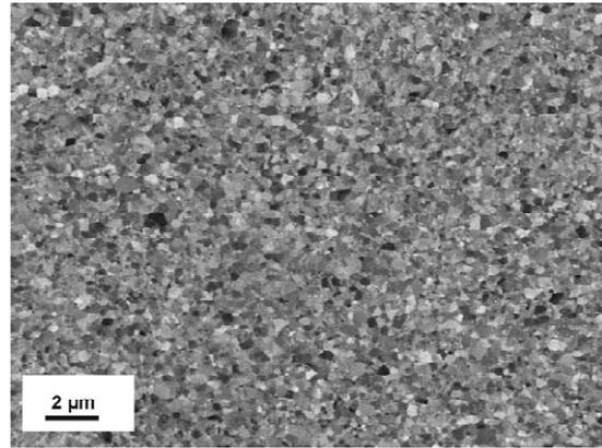
**Fig. 1.** (a) Definition of the direction of observation, (b) the microstructure of the bulk Ni sample HPT deformed at room temperature to an equivalent shear strain  $\varepsilon_{\text{VHPT}}$  of 32 observed in tangential direction.
