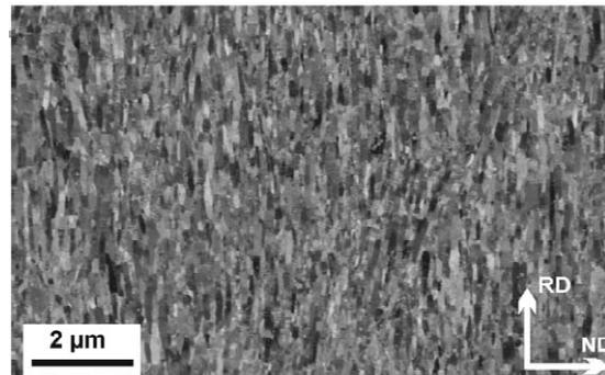
**Fig. 2.** (a) The microstructures of the bulk Ni sample which were additionally cold rolled after HPT deformation with 83% reduction and (b) with 96% reduction. The rolling direction (RD) and normal direction (ND) during the cold rolling is depicted in the lower right corner.
