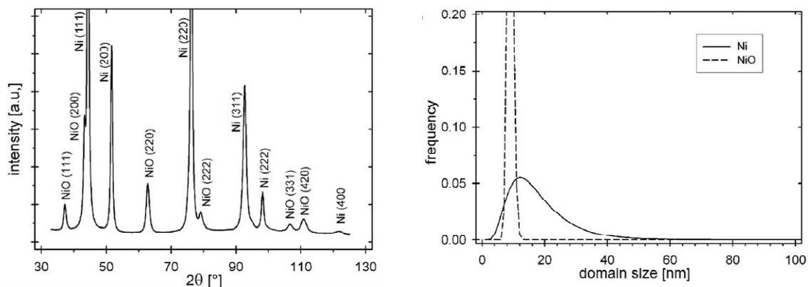
**Fig. 5.** (a) XRD pattern of HPT consolidated sample of oxidized Ni powder, (b) size distribution of the coherently scattering domains as determined by multiple X-ray Bragg profile analysis.
