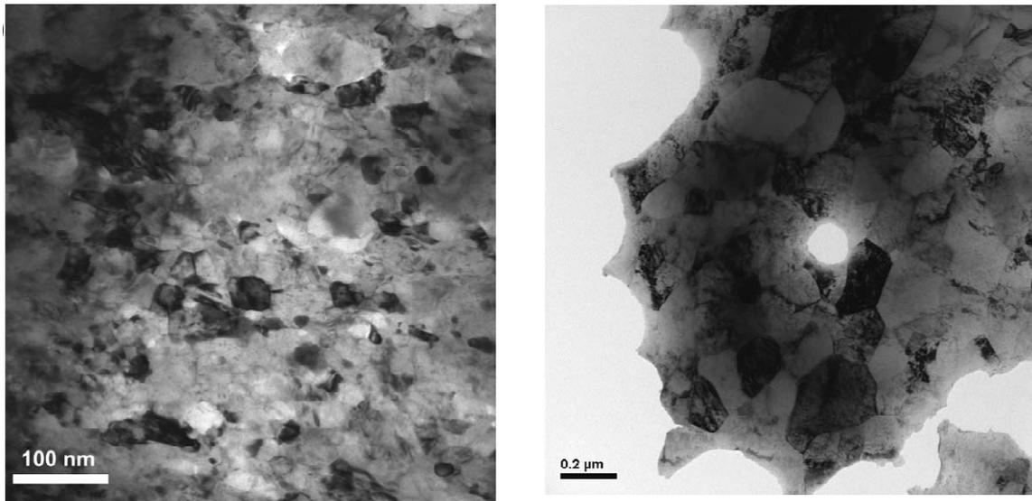
**Fig. 4.** (a) Bright-field transmission electron micrograph of the microstructure of the HPT consolidated sample of oxidized Ni powder [18], (b) bright-field transmission electron micrograph of the microstructure of the HPT deformed sample of bulk Ni. Please note the difference in magnification.
