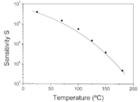
**Fig. 6.** Sensitivity of a 100nm thick InO<sub>x</sub> film vs. temperature. The line is a guide to the eyes.
