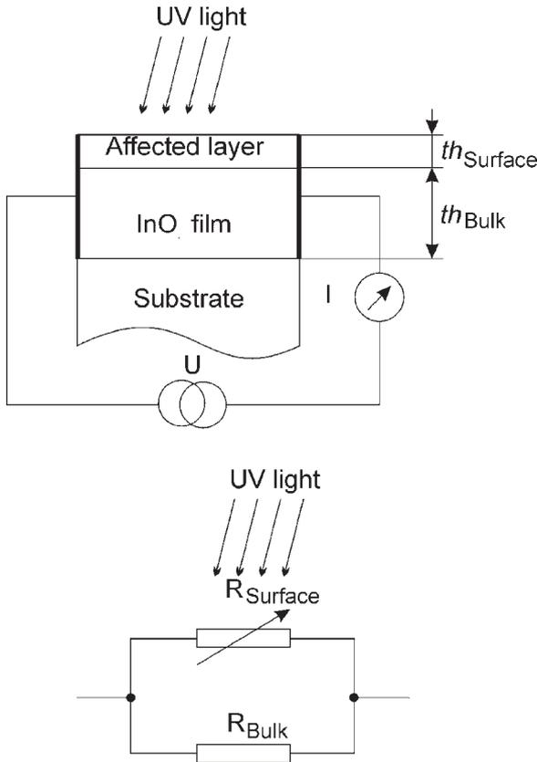
Fig. 1. Resistor model of the UV-irradiated  $\text{InO}_x$  film.
