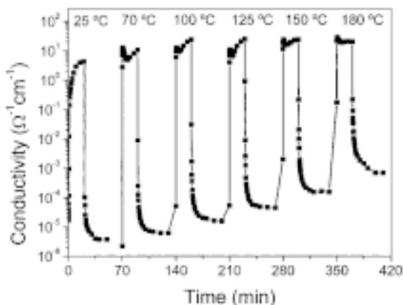
**Fig. 2.** Photoreduction and subsequent oxidation of a 100 nm thick InO<sub>x</sub> film deposited at RT measured at different temperatures.
