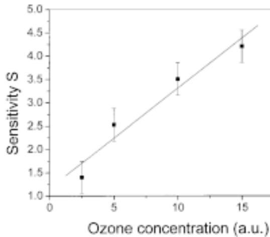
Fig. 7. Response of films to different concentrations of ozone measured at RT.
