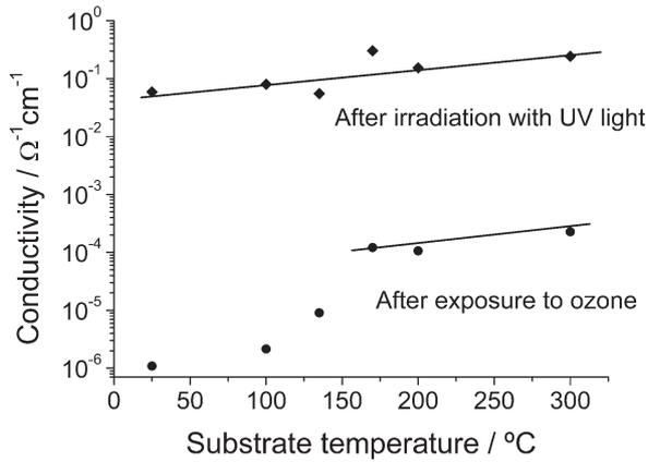
**Fig. 4.** Maximum and minimum conductivities of  $\text{InO}_x$  films deposited at different substrate temperatures.
