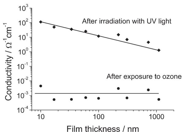
**Fig. 3.** Maximum and minimum conductivities of InO<sub>x</sub> films as a function of film thickness.
