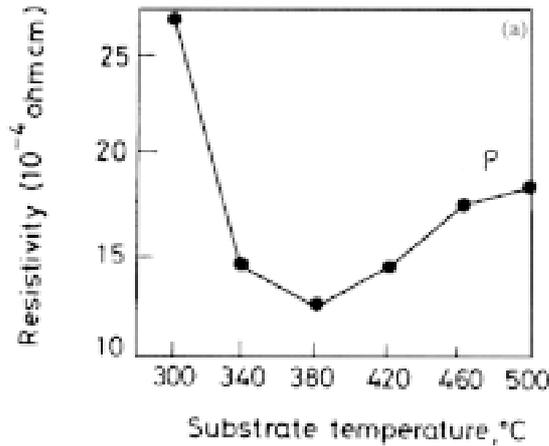
**Fig. 5.** Variation of resistivity of In<sub>2</sub>O<sub>3</sub> films with different substrate temperatures (Ref. [45]).
