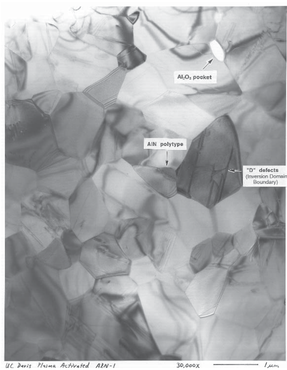
Fig. 4. Regular (left) and high resolution TEM (right) of field sintered AlN.
