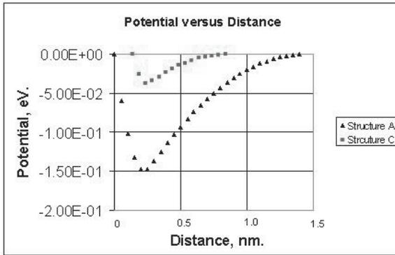
**Fig.3.** Potential profiles for Structure A (asymmetric) and Structure C (symmetric).
