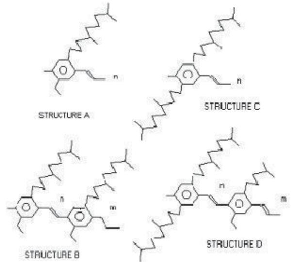
**Fig.1.** Different conjugated and partially conjugated OC<sub>1</sub>C<sub>10</sub>PPV [10].
