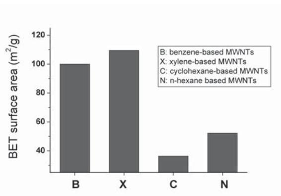
**Fig. 3.** BET surface area of the four as-synthesized MWNTs.
