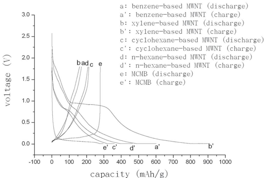
**Fig. 2.** First cycle charge-discharge plots for different precursor-based MWNTs.
