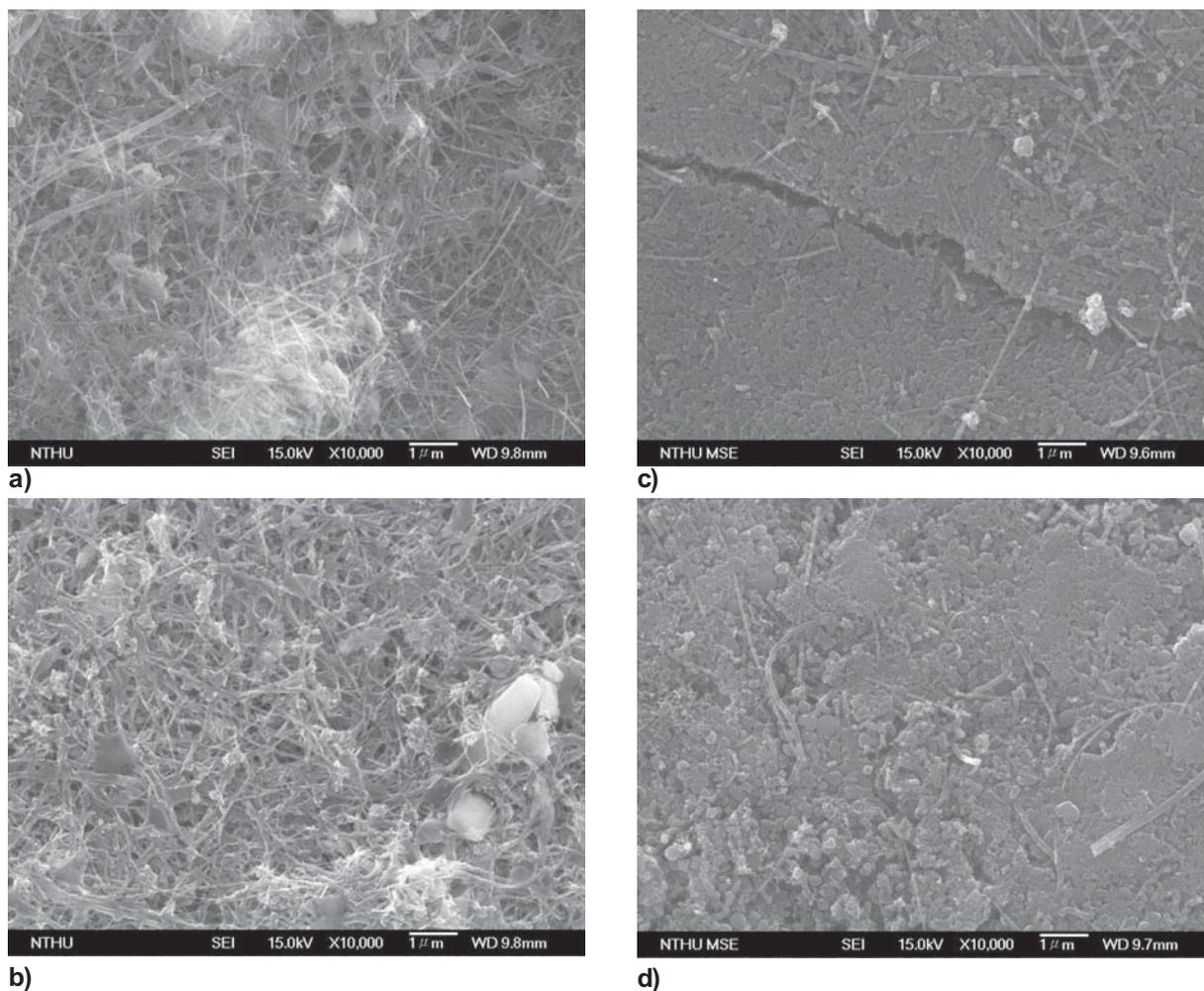
**Fig. 1.** (a) SEM image of as-prepared benzene-based MWNT electrode before the first charge-discharge cycle (10K); (b) SEM image of as-prepared xylene-based MWNT electrode before the first charge-discharge cycle (10K); (c) SEM image of as-prepared cyclohexane-based MWNT electrode before the first charge-discharge cycle (10K); (d) SEM image of as-prepared n-hexane-based MWNT electrode before the first charge-discharge cycle (10K).
