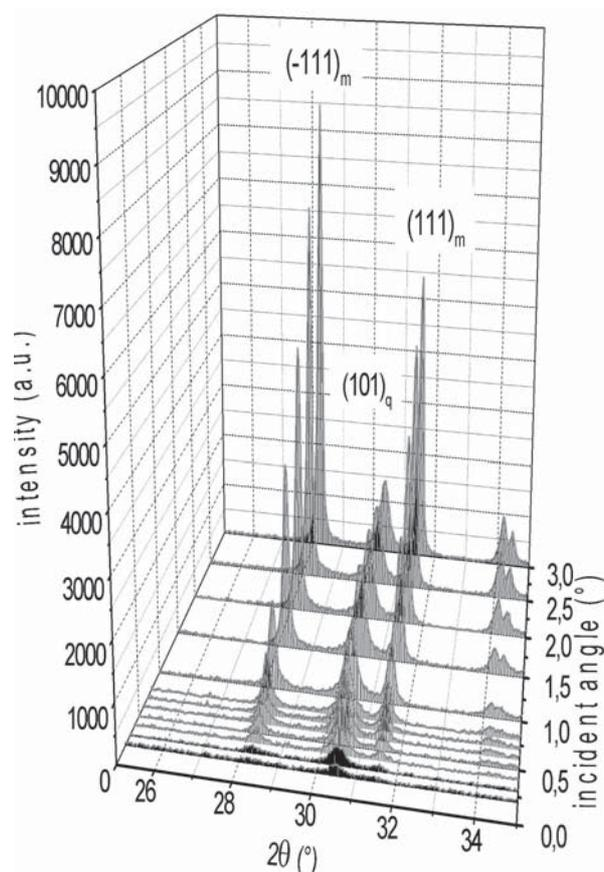
**Fig. 1.** Zoom of X-ray diffraction diagrams collected on irradiated zirconia samples at different incidence angles (*i.e* depths). Between two monoclinic Bragg peaks, a new peak associated to the tetragonal phase appears on irradiated samples. The saturation of the intensity of this peak suggests that the tetragonal phase is localized in the damaged area.
