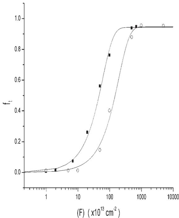
**Fig. 3.** Evolution of the tetragonal volume fraction of zirconia versus the fluence for different incident ions (black squares for 800 keV Bi and open dots for 400 keV Xe). Simple kinetic equations (full lines) fit experimental data.
