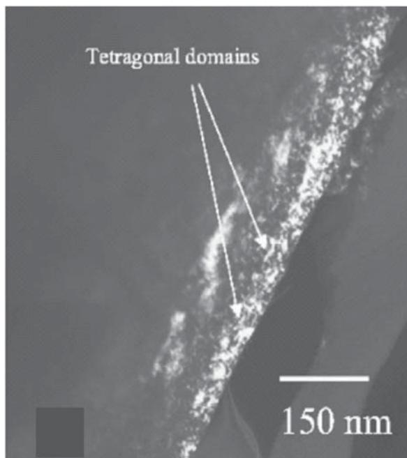
**Fig. 2.** Dark field image on the most irradiated zirconia samples. The dark field exhibits nanometric tetragonal domains. The size of these domains is similar to the one extracted from X-ray diffraction and is about 10 nm.
