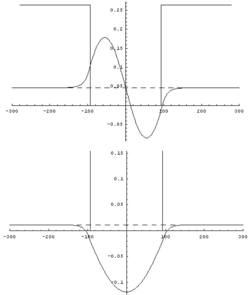
**Fig. 2.** NHI optimised effective QW hosting the fundamental (lower) and first excited (upper) 2DEG wavefunction, with the respective energy eigenvalue marked and the wave-function penetration length traceable.
