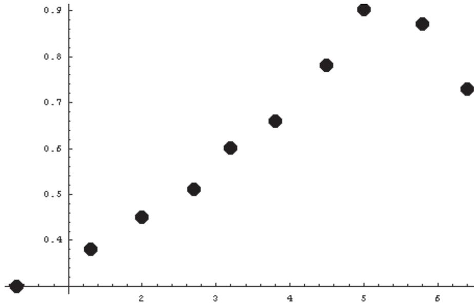
**Fig. 1.** Reduced PPE  $\Delta\mu/\mu_0$  in the NHI 2DEG mobility  $\mu$  versus the decimal logarithm  $\log(\delta/\delta_0)$  of the reduced incoming cumulative photon dose.
