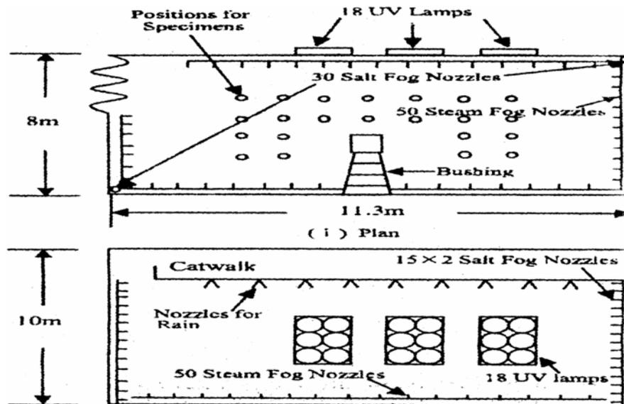
Fig. 6. 275 kV full scale insulator test chamber.
