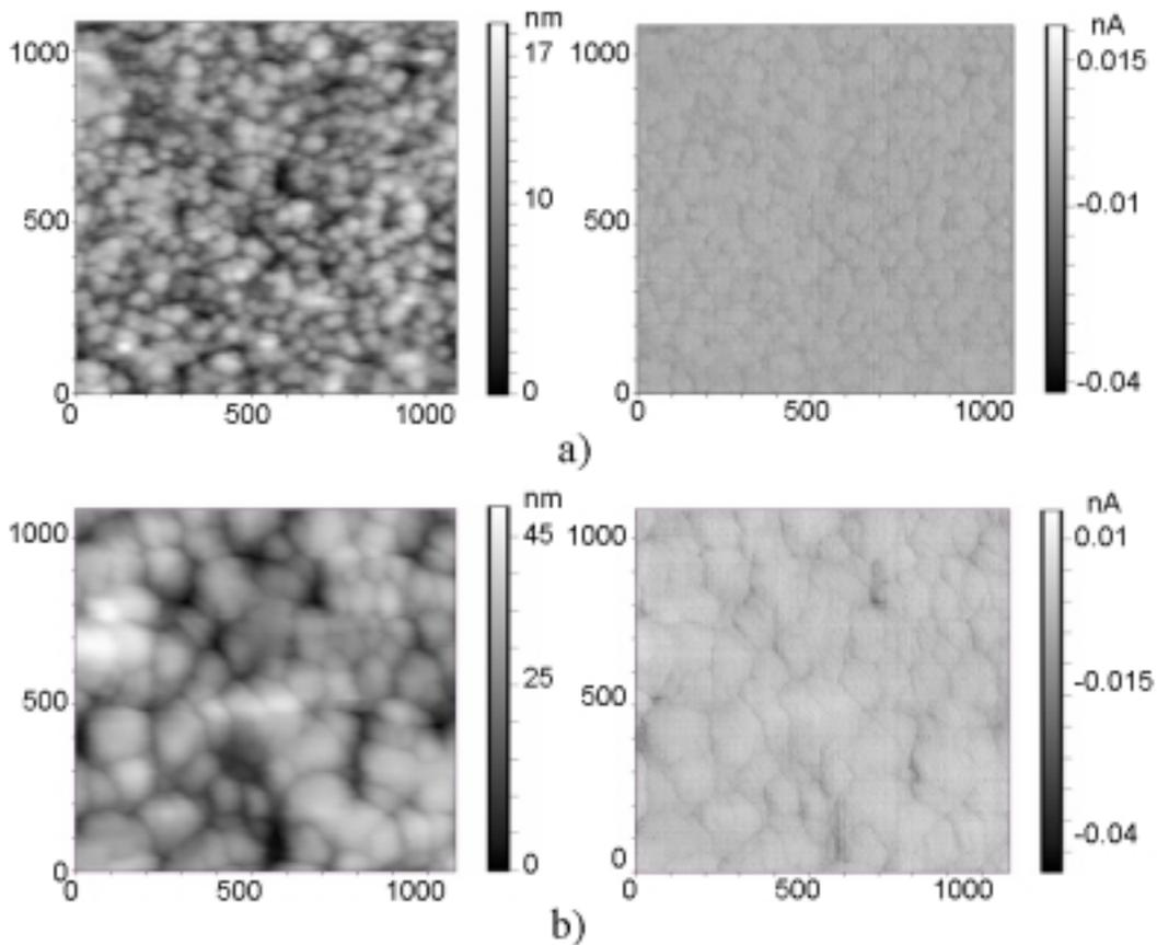
**Fig. 4.** Surface topography (left) and lateral force images (right) with scanned area ( $1 \times 1$ )  $\mu\text{m}$  for NN on a) Pt/SRO, and b) Si/SRO. The RMS roughness for the given images is 3 and 8 nm.
