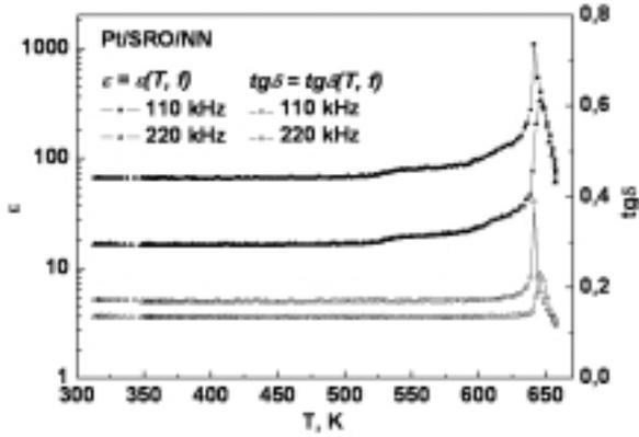
**Fig. 2.** Dielectric permittivity  $\varepsilon$  (solid symbols) and loss factor  $\text{tg}\delta$  (open symbols) as the function of the temperature at frequencies of 110 kHz and 220 kHz.
