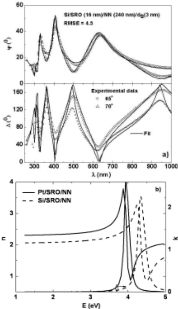
**Fig. 5.** Experimental main ellipsometric angles  $\psi$  and  $\Delta$  (open symbols) and their numerical fit (solid line) as a function of wavelength at two incident angles for the Si/SRO/NN sample (a); refractive coefficient  $n$  (the left axis) and extinction coefficient  $k$  (the right axis) of NN films deposited on Pt/SRO (solid line) and Si/SRO (dashed line) substrates (b).
