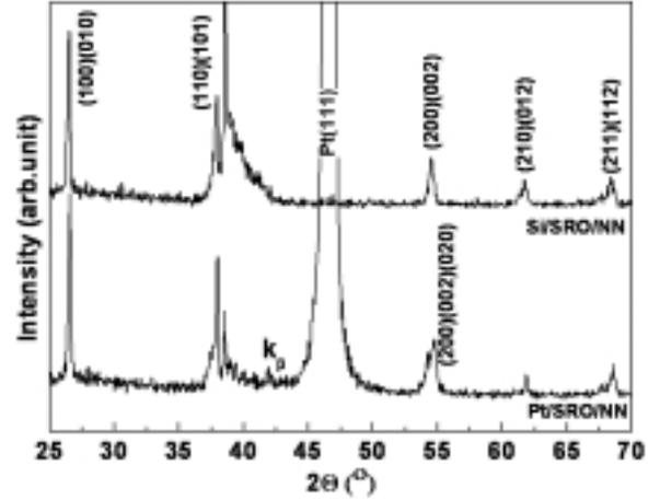
**Fig. 1.** X-ray diffraction studies using  $2\theta$  scans for NN thin films on 2 different substrates - Pt/SRO and Si/SRO.
