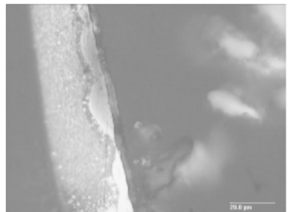
Fig. 5. Optical micrograph of ACY1 (ribbon etched with aqua regia).
