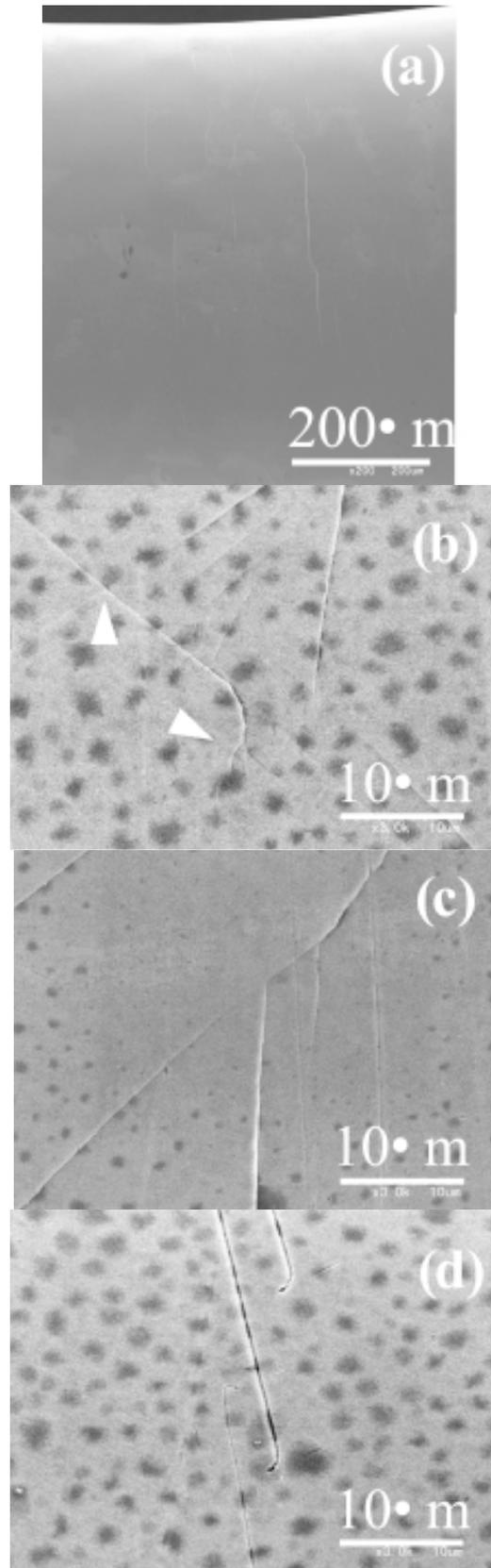
**Fig. 2.** Specimen surface morphology in the Ti-based BMG after  $N=6 \cdot 10^6$  cycles of  $2\sigma_a/\sigma_w=0.98$ . (a) Macroscopic morphology of shear bands, and (b)–(d) examples of the kink, branch, intersection, and rotate in shear bands.
