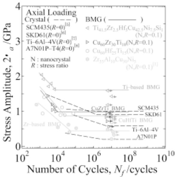
**Fig. 1.** Comparison between the fatigue strength of the BMGs and crystalline alloys.
