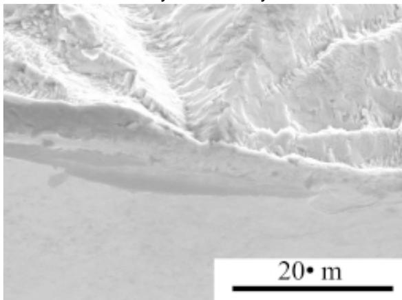
**Fig. 3.** Fracture and specimen surface morphology near the fatigue crack initiation region in the Ti-based BMG.
