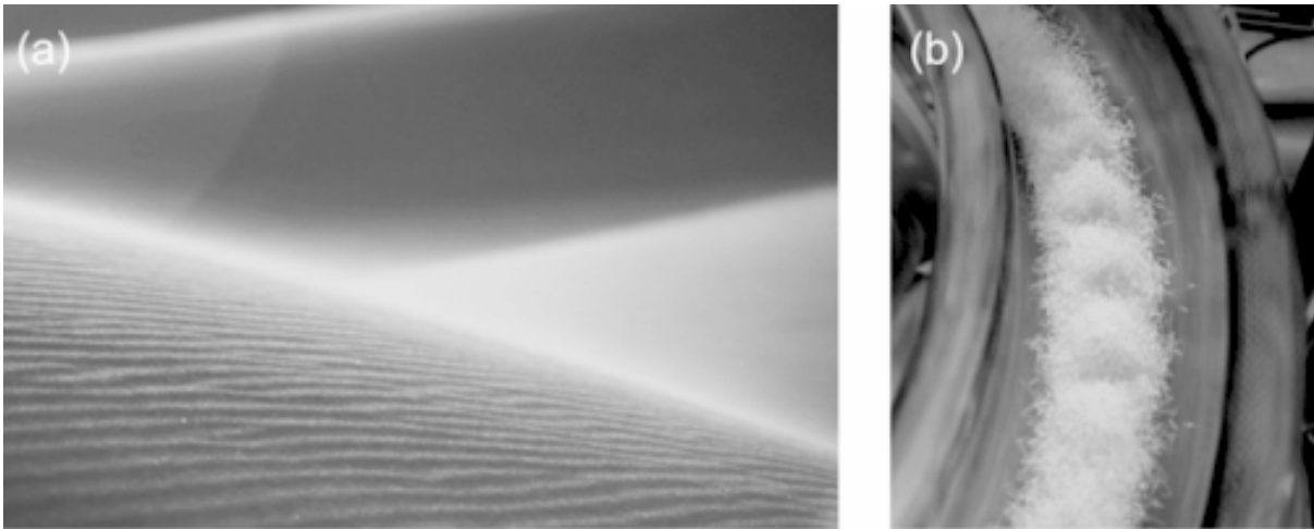
Fig. 1. (a) Sand dune decorated with aeolian ripples, Great Sand Dunes National Monument, Colorado, USA, (b) Oscillating granular surface wave on a vibratory conveyor.
