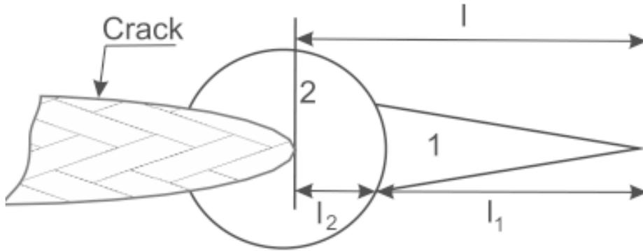
**Fig. 1.** Pre-fracture zone. 1 is the area of elastic deformations, 2 is the area of plastic deformations. Total length of influence zone  $l$  is the sum of elastic and plastic parts.
