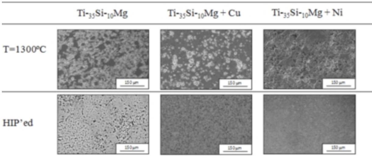
**Fig. 4.** Morphology of the coated and uncoated Ti-35Si-10Mg samples sintered at 1300 °C and HIP'ed.
