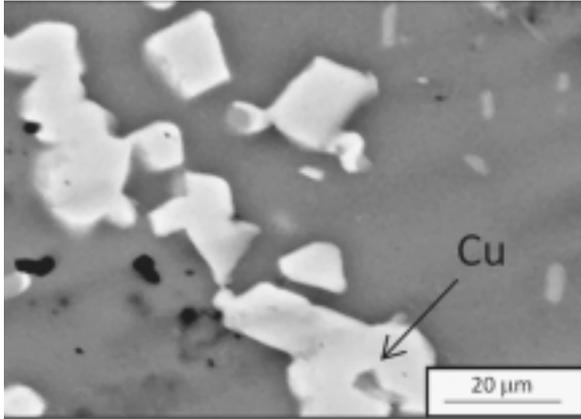
**Fig. 5.** Morphology (BSE-SEM image) of the Ti-35Si-10Mg-Cu HIP'ed sample showing segregation of Cu.
