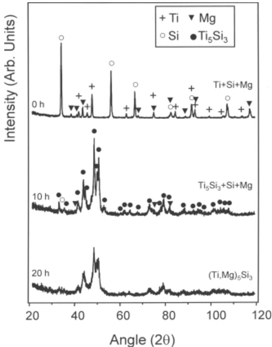
Fig. 2. XRD patterns of the Ti-35Si-10Mg mixture as a function of milling time.
