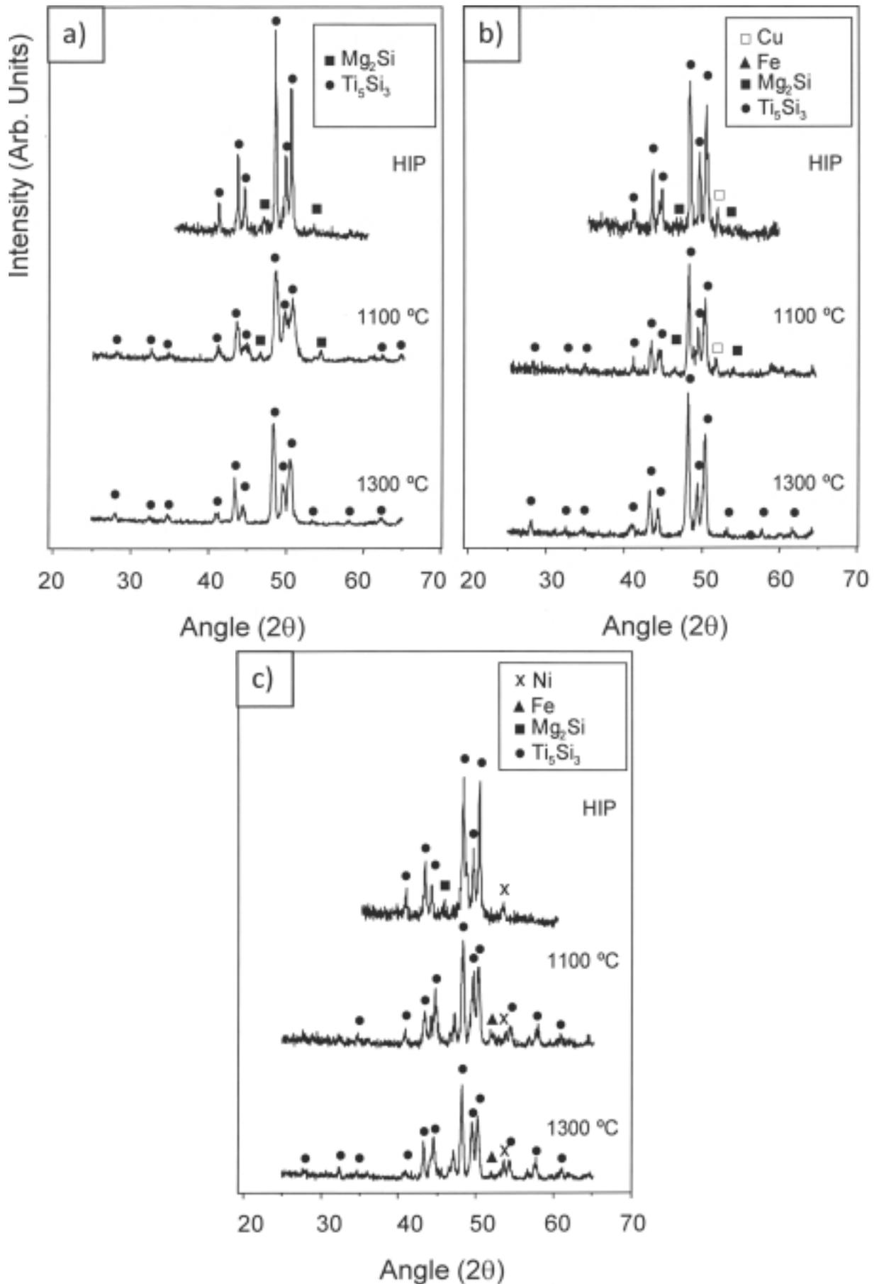
**Fig. 6.** XRD patterns of the uncoated (a), Cu-coated (b) and Ni-coated (c) Ti-35Si-10Mg samples sintered at two different temperatures and HIP'ed.
