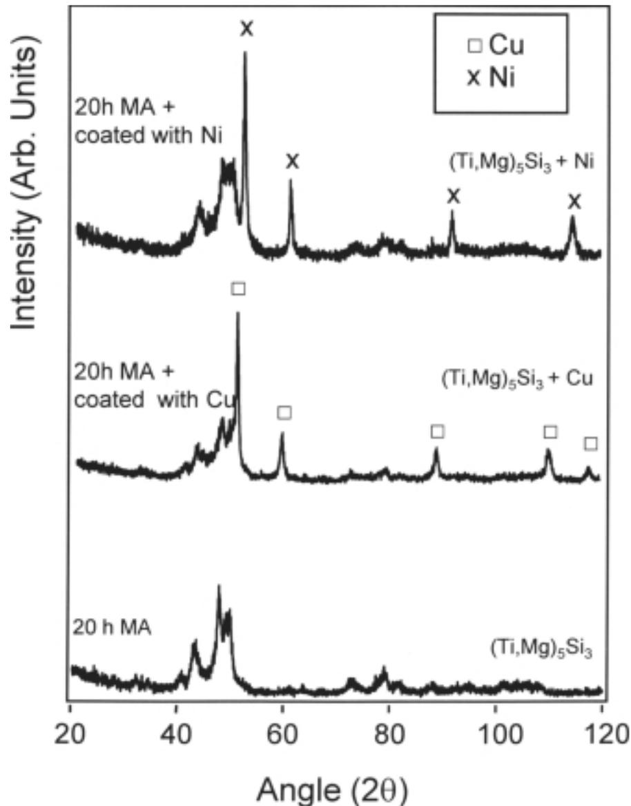
Fig. 3. XRD patterns of the coated and uncoated Ti-35Si-10Mg mixture milled for 20h.
