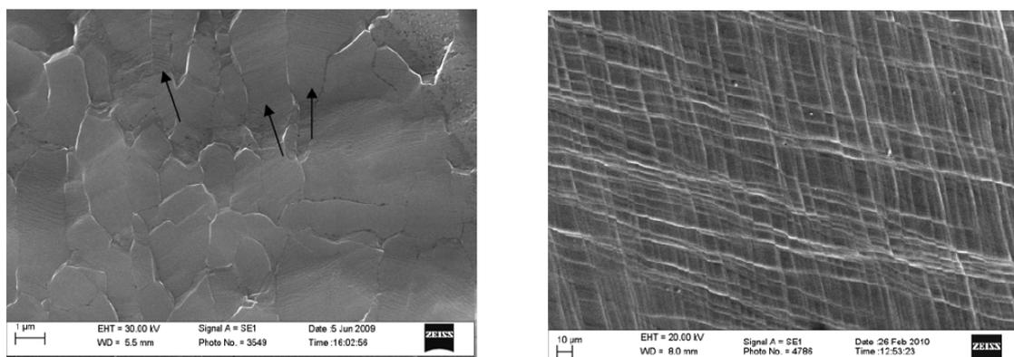
**Fig. 3.** SEM images of deformation relief on the polished surface of the sample 3 at the origin of the neck (a) and that of the recrystallized aluminum sample (b). The sliding between grains and intragrain dislocation slip steps are visible in (a). Black arrows indicate glide lines.
