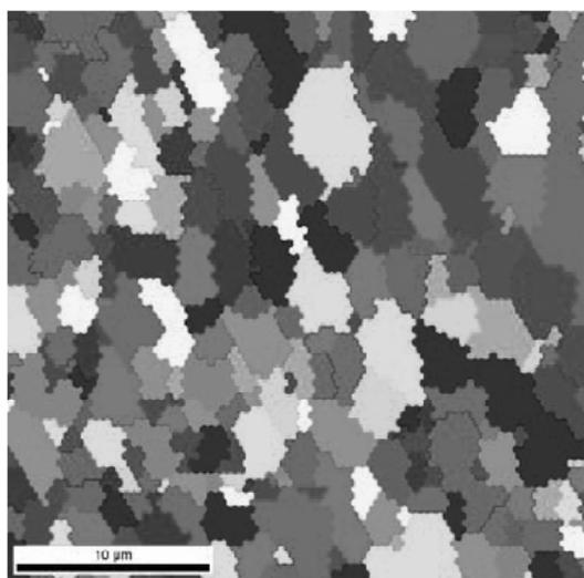
**Fig. 4.** OIM map of subgrain structure obtained for the scan 3 on the sample 5. The same scan as in Fig. 5b.
