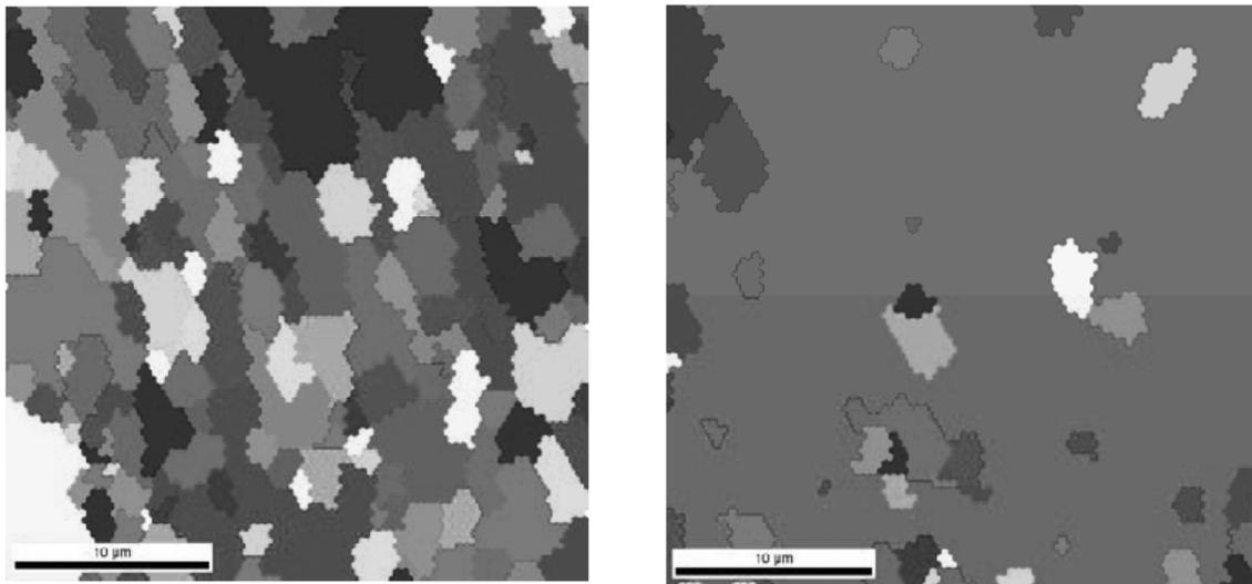
**Fig. 5.** OIM maps of grain structure obtained on the sample 5 for the scans 2 (a) and 3 (b). Compare Figs. 5b and 4 representing the difference of grain and subgrain structure on the same scan.
