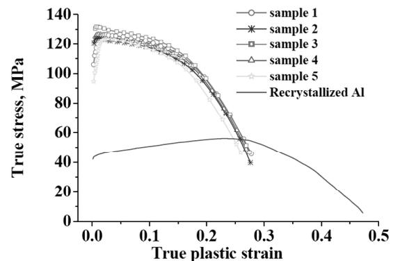
Fig. 2. The true plastic flow curves obtained for the test samples corresponding to the different distance from the top surface of the billet. Compare with the flow curve obtained for recrystallized aluminum.
