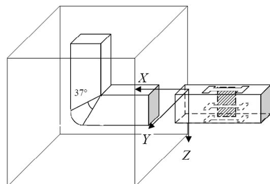
**Fig. 1.** The scheme illustrated the position of the system of coordinates and how the tensile samples and the sample for microhardness measurements were cut. The latter sample is marked by hatching.
