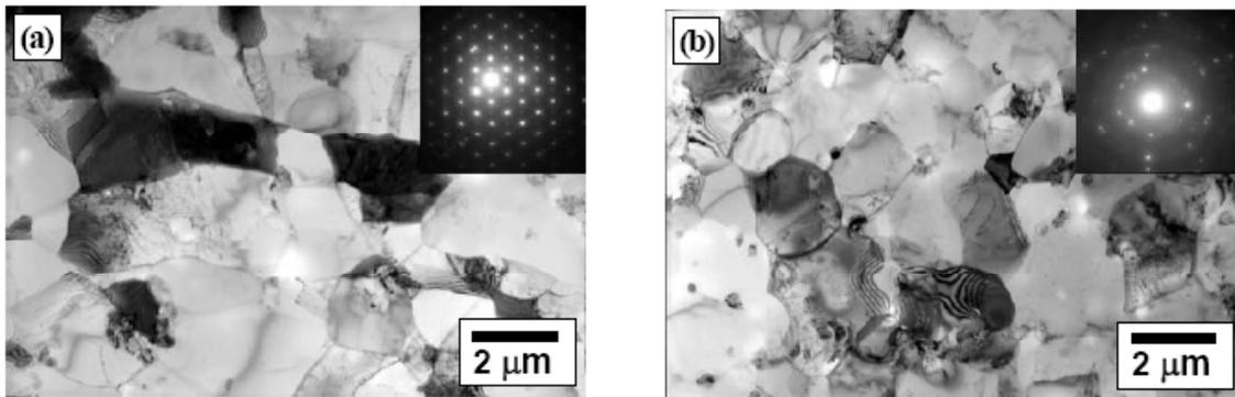
**Fig. 2.** Typical TEM micrographs of the ECAE substructures evolved in a 1421 alloy; (a) one pass and (b) eight passes. The electron diffraction patterns were obtained from the selected areas of 10  $\mu\text{m}$  in diameter.
