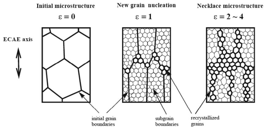
**Fig. 5.** Schematic drawing of the structural changes taking place in a 1421 alloy during hot ECAE.
