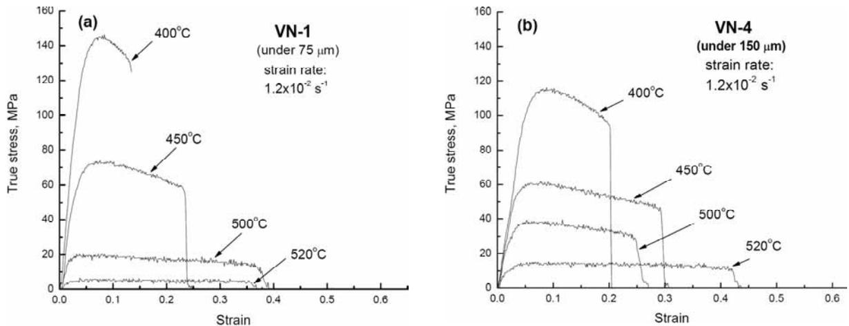
**Fig. 2.** Temperature change of stress-strain curves of VN-1 and VN-4 alloys. (a) VN-1 alloy produced from the powder under 75  $\mu\text{m}$  in size, (b) VN-4 alloy from the powder under 150  $\mu\text{m}$ .
