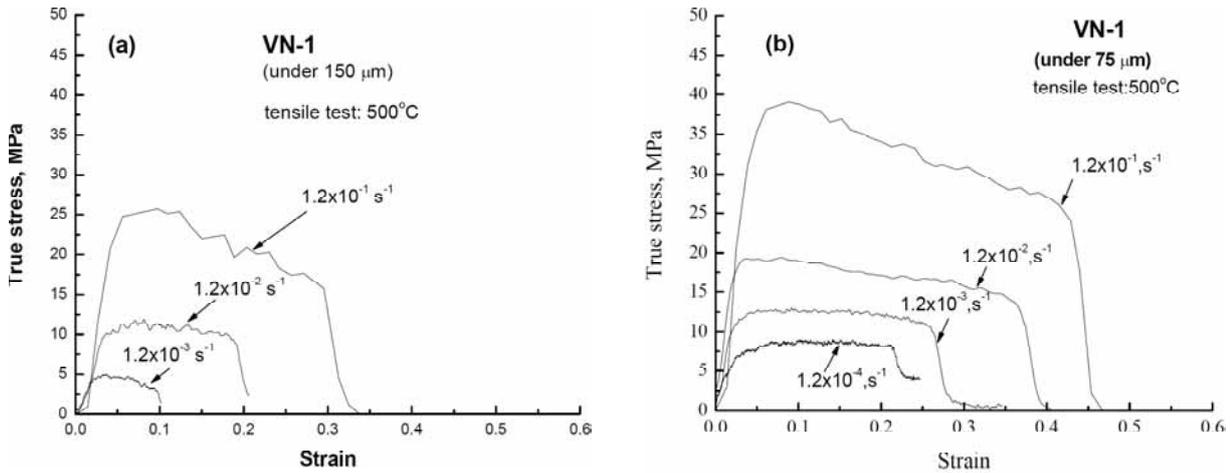
**Fig. 4.** Change of stress-strain curves of VN-1 alloy by strain rate. (a) for powder under 150  $\mu\text{m}$  in size, (b) for under 50  $\mu\text{m}$ .
