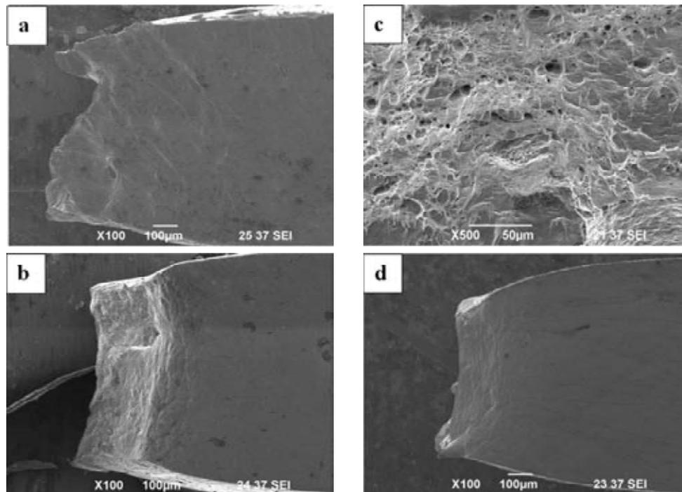
**Fig. 5.** Fracture morphology after tensile tests of (a) UFG<sub>1pECAP+HSRD</sub> Cu, (b) UFG<sub>4pECAP+HSRD</sub> Cu, (c) high magnification of UFG<sub>4pECAP+HSRD</sub> Cu, (d) UFG<sub>8pECAP+HSRD</sub> Cu.
