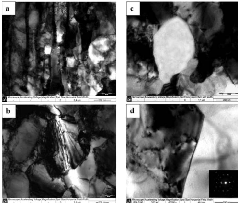
**Fig. 4.** TEM microstructures for  $\text{Cu}_{4\text{pECAP+HSRD}}$ : (a) lamellar dislocation bands (LBs), (b) dislocations in grains and boundaries, (c) recrystallized grain, (d) a boundary of recrystallized grain and the selected area diffraction pattern.
