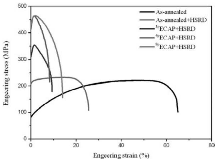
Fig. 1. Engineering stress-strain curves for as-annealed, as-annealed and ECAP Cu after HSRD.
