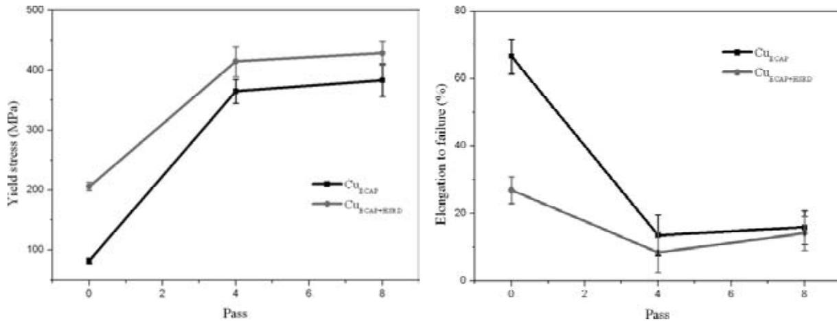
**Fig. 2.** The mechanical behaviors of Cu<sub>ECAP</sub> and Cu<sub>ECAP+HSRD</sub> samples vs. different number ECAP passes. (a) yield stress, (b) elongation to failure.
