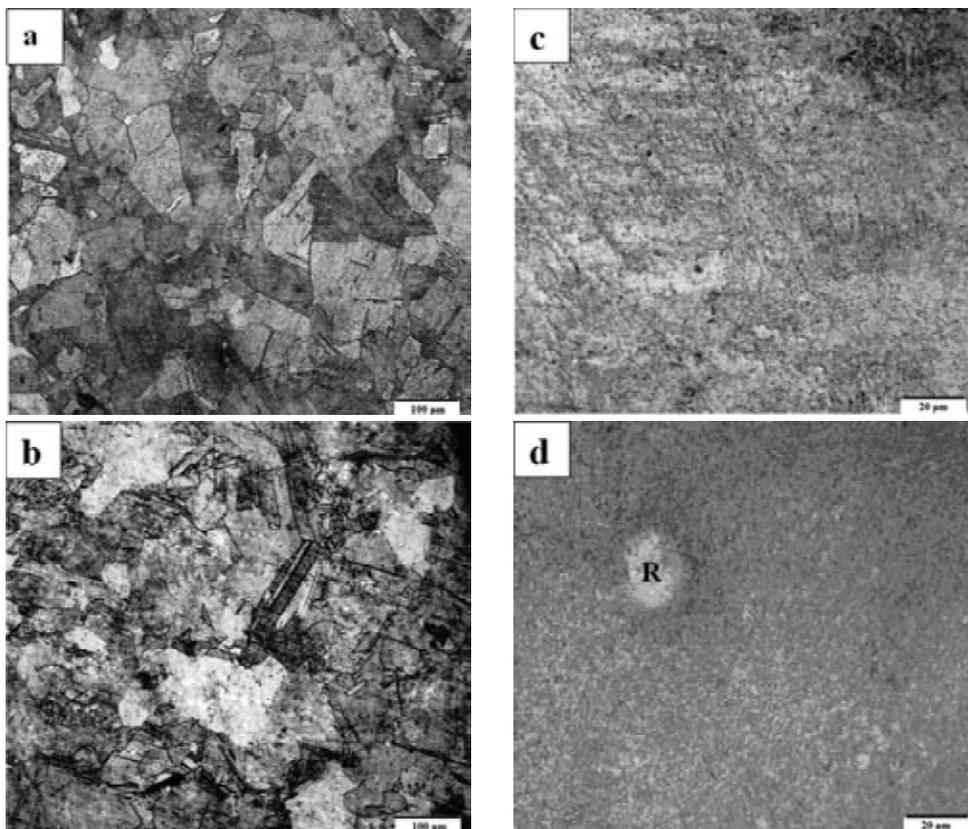
**Fig. 3.** Optical microscopy images: (a) CG Cu, (b) CG<sub>HSRD</sub> Cu, (c) Cu<sub>4pECAP+HSRD</sub>, (d) Cu<sub>8pECAP+HSRD</sub>.
