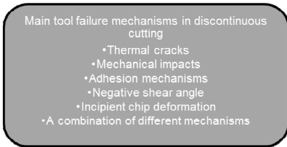
**Fig. 2.** Failure mechanisms on discontinuous cutting.
