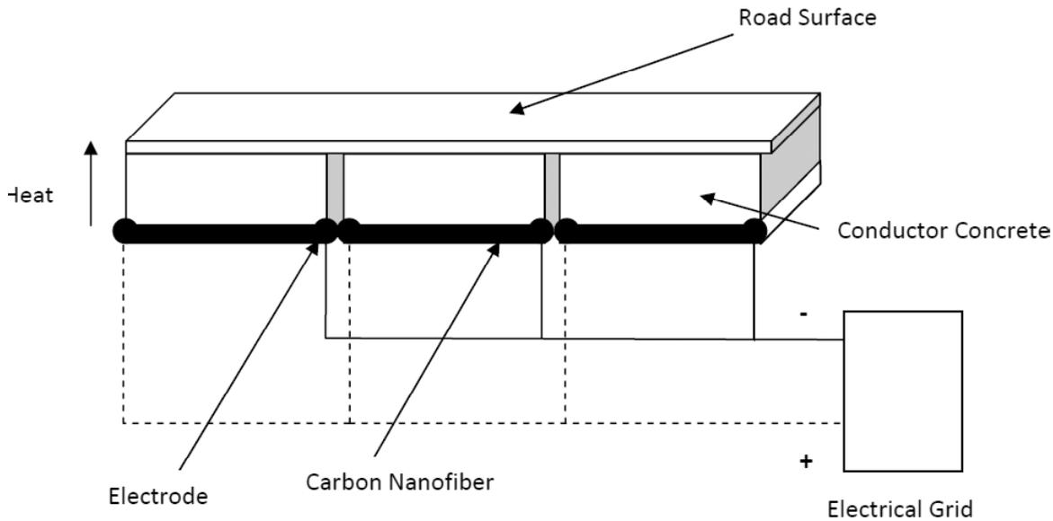
**Fig. 3.** Mechanism of self heating concrete.
