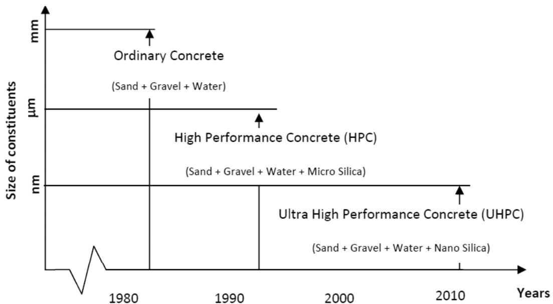
Fig. 1. Evolution of concrete from millimeter to nanometer era.
