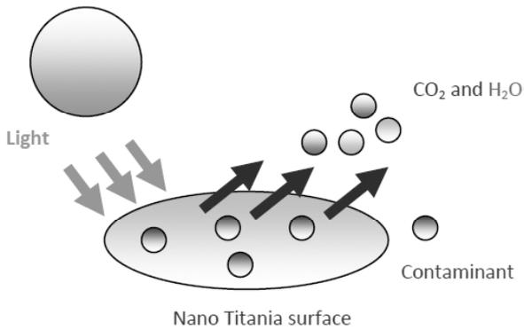
**Fig. 2.** Mechanism of nano titania photocatalysis.
