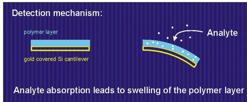
Fig. 3. Cantilever detection mechanism [IBM – Zurich].
