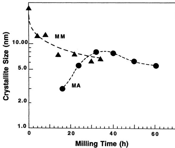
**Fig. 3.** Crystallite size for FeTi intermetallic phase for low energy mechanical alloying of Fe and Ti powders (solid circles), and mechanical milling of the FeTi compound powders (solid triangles) [21].
