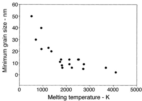
**Fig. 1.** Minimum nanocrystalline grain size for ball milled elements vs. their melting temperature. Data from references 7, 9, 10, 11.
