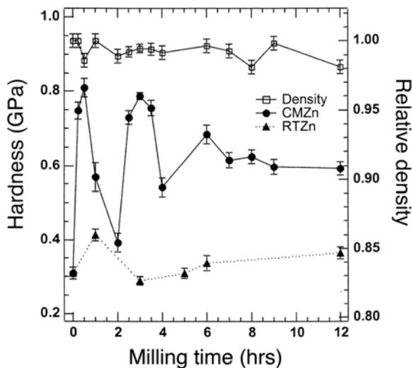
**Fig. 2.** Hardness vs. milling time for cryomilled Zn (solid circles) and Zn milled at room temperature (solid triangles). The relative density for the cryomilled samples is shown by the open squares. Reference 19.
