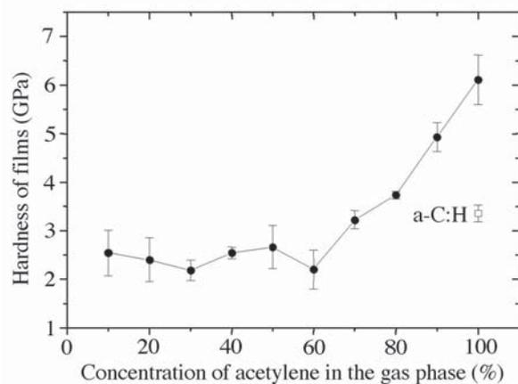
**Fig. 5.** Hardness of : (●) Cu/a-C:H films and (□) a-C:H films prepared by plasma-enhanced chemical vapor deposition from pure  $C_2H_2$  as a function of the  $C_2H_2$  concentration in the gas phase.
