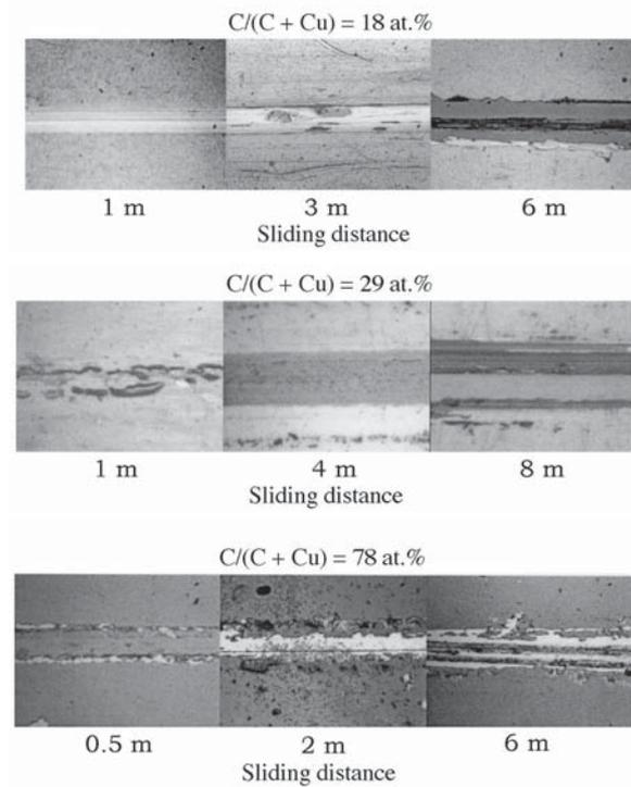
**Fig. 8** Optical micrographs of wear tracks for Cu/a-C:H films with a carbon content of : (a) 18 at.%, (b) 29 at.%, and (c) 78 at.% after various sliding distances.
