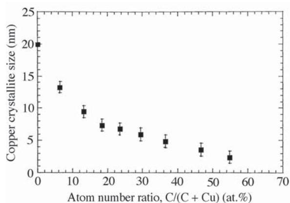
**Fig. 2.** Size of smallest copper crystallites embedded in the carbon matrix versus carbon content of films.
