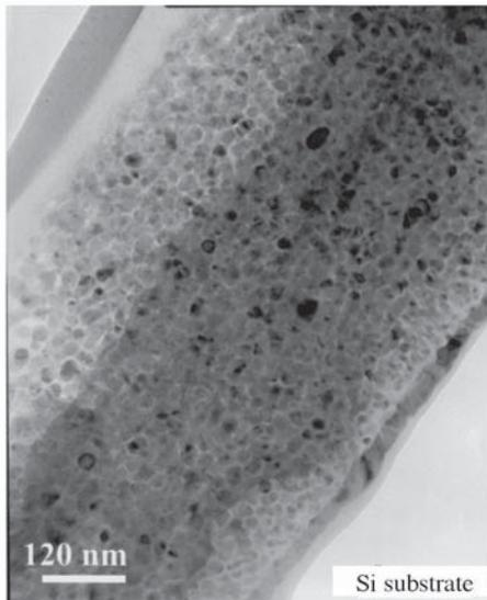
**Fig. 3.** Typical transmission electron micrograph on the cross-section of a Cu/a-C:H film deposited from a gas mixture containing 20% of acetylene.
