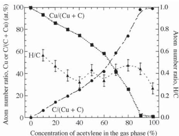
**Fig. 1.** Composition of Cu/a-C:H composite films versus  $C_2H_2$  concentration in the gas phase.
