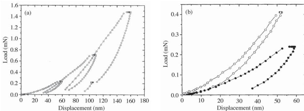
**Fig. 6.** a) Load-displacement curves of Cu/a-C:H films deposited from a gas mixture containing 60% of  $C_2H_2$ . The large hysteresis loops are characteristic of a soft polymer-like a-C:H matrix. b) First loading cycle for Cu/a-C:H films produced from a gas mixture containing: (●) 60% of  $C_2H_2$  and (○) 100% of  $C_2H_2$ . The small hysteresis loop is characteristic of an ion-hardened a-C:H matrix.
