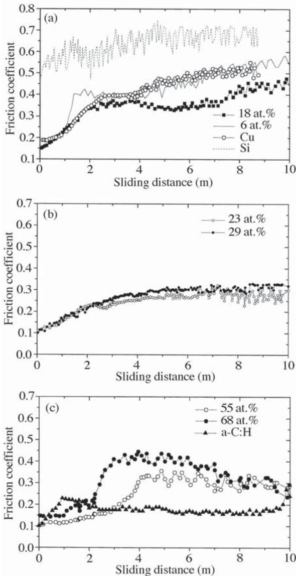
**Fig. 7.** Friction coefficient versus sliding distance for various samples: (a) bare Si substrate, pure Cu film and Cu/a-C:H films containing 6 and 18 at.% of carbon, (b) Cu/a-C:H films containing 23 and 29 at.% of carbon, and (c) a-C:H film prepared by plasma-assisted chemical vapor deposition from pure  $C_2H_2$  and Cu/a-C:H films containing 55 and 68 at.% of carbon.
