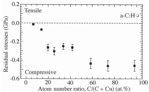
**Fig. 4.** Residual stresses developed in: (○) a-C:H films prepared by plasma-assisted chemical vapor deposition from pure  $C_2H_2$  and (●) Cu/a-C:H films as a function of the carbon content in the films.
