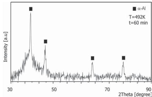
**Fig. 7.** X-Ray pattern of  $\text{Al}_{88}\text{Mm}_4\text{Ni}_5\text{Fe}_3$  alloy after isothermal annealing at 492K for 60 min.
