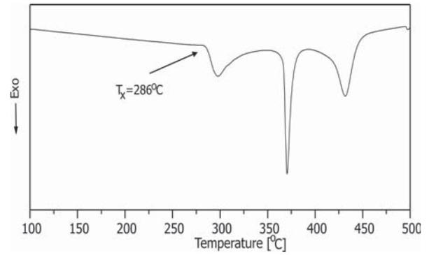
Fig. 2. DSC curve of  $\text{Al}_{88}\text{Mm}_4\text{Ni}_5\text{Co}_3$  alloy.
