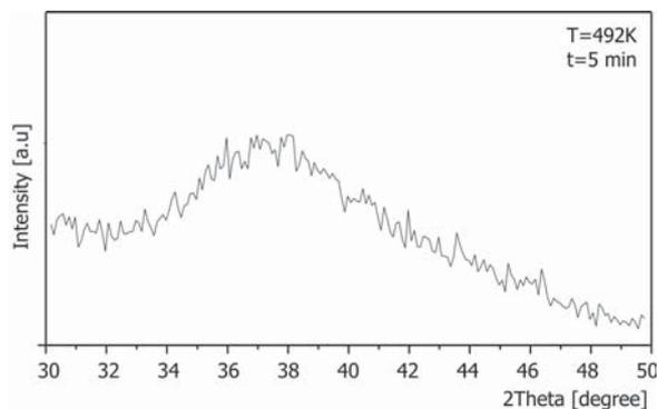
Fig. 3. X-Ray pattern of amorphous  $\text{Al}_{88}\text{Mm}_4\text{Ni}_5\text{Fe}_3$  alloy.
