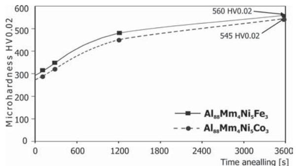
**Fig. 9.** Dependence of the microhardness on the annealing time of nanocrystalline  $\text{Al}_{88}\text{Mm}_4\text{Ni}_5(\text{Co}, \text{Fe})_3$  alloys.
