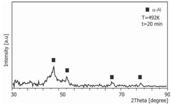
**Fig. 6.** X-Ray pattern of  $\text{Al}_{88}\text{Mm}_4\text{Ni}_5\text{Co}_3$  alloy after isothermal annealing at 492K for 20 min.
