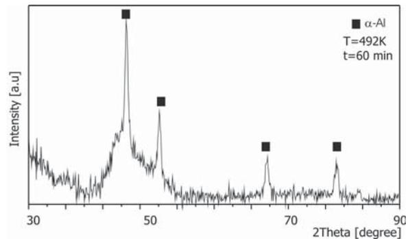
**Fig. 8.** X-Ray pattern of  $\text{Al}_{88}\text{Mm}_4\text{Ni}_5\text{Co}_3$  alloy after isothermal annealing at 492K for 60 min.
