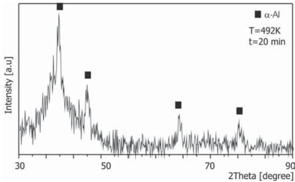
**Fig. 5.** X-Ray pattern of  $\text{Al}_{88}\text{Mm}_4\text{Ni}_5\text{Fe}_3$  alloy after isothermal annealing at 492K for 20 min.
