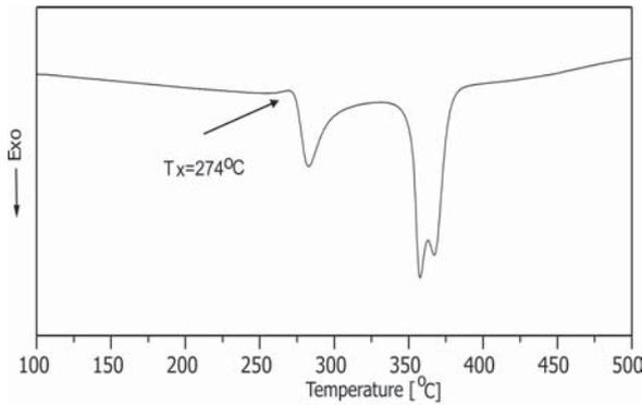
Fig. 1. DSC curve of  $\text{Al}_{88}\text{Mm}_4\text{Ni}_5\text{Fe}_3$  alloy.
