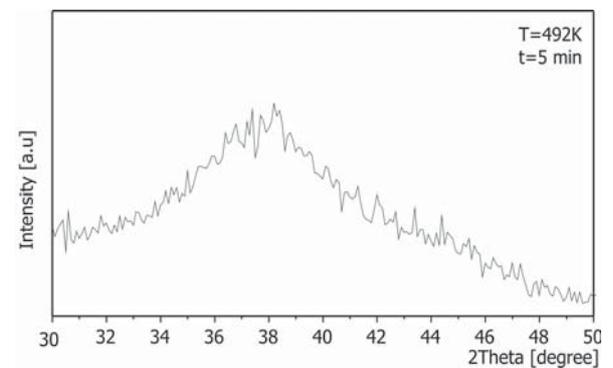
Fig. 4. X-Ray pattern of amorphous  $\text{Al}_{88}\text{Mm}_4\text{Ni}_5\text{Co}_3$  alloy.
