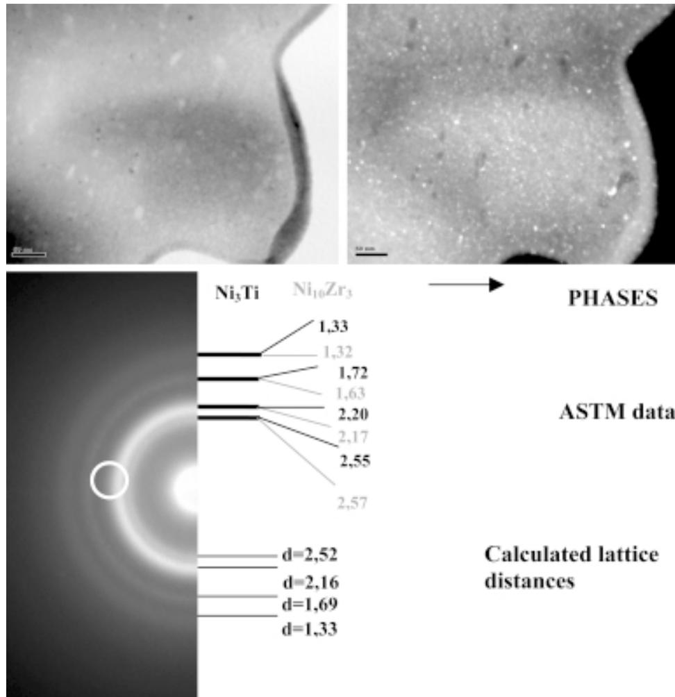
**Fig. 8.** UHP compacted milled powder of alloy B (a) TEM Bright field, (b) Dark field and (c) Selected area electron diffraction pattern with marked positions  $Ni_3Ti$  of and  $Ni_{10}Zr_3$  phases diffraction lines positions.
