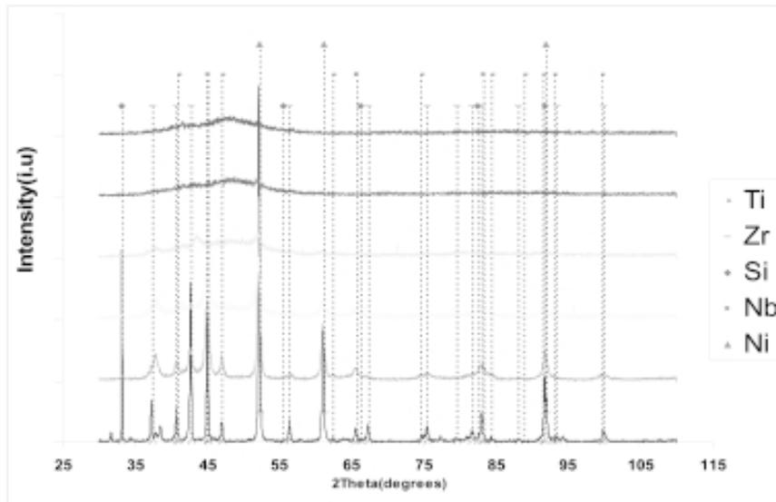
Fig. 5. X-Ray diffraction curves of alloy C powder after indicated milling times.
