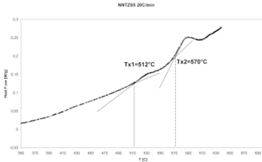
**Fig. 2.** DSC Analysis of Ni<sub>45</sub>-Nb<sub>21</sub>-Ti<sub>16</sub>-Zr<sub>13</sub>-Si<sub>5</sub> (alloy B) ribbon.
