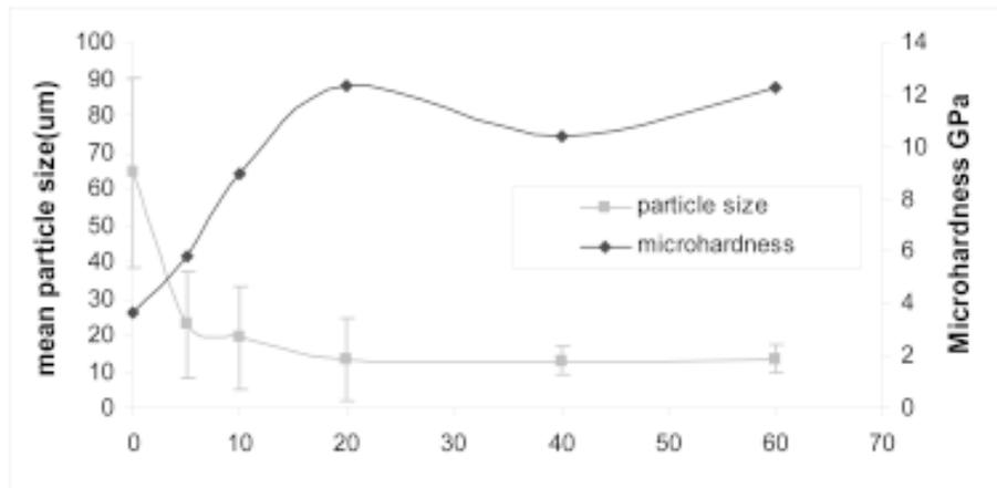
Fig. 6. Mean particle size and microhardness changes during milling time of the alloy C.
