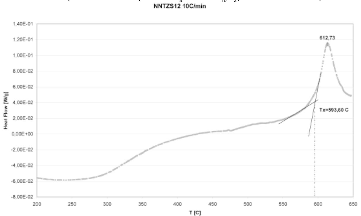
**Fig. 9.** DSC curve of UHP compacted sample of the alloy C.
