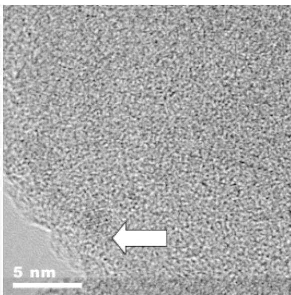
**Fig. 4.** HRTEM microstructure of Ni<sub>50,34</sub>-Nb<sub>14,38</sub>-Ti<sub>17,32</sub>-Zr<sub>15,15</sub>-Si<sub>2,81</sub> (at. %) (alloy C) ribbon cast at the linear drum rate of 8 m/sec.
