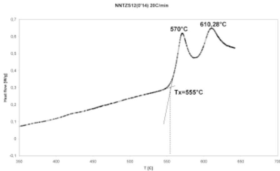
**Fig. 3.** DSC Analysis of Ni<sub>50,34</sub>-Nb<sub>14,38</sub>-Ti<sub>17,32</sub>-Zr<sub>15,15</sub>-Si<sub>2,81</sub> (alloy C) ribbon.
