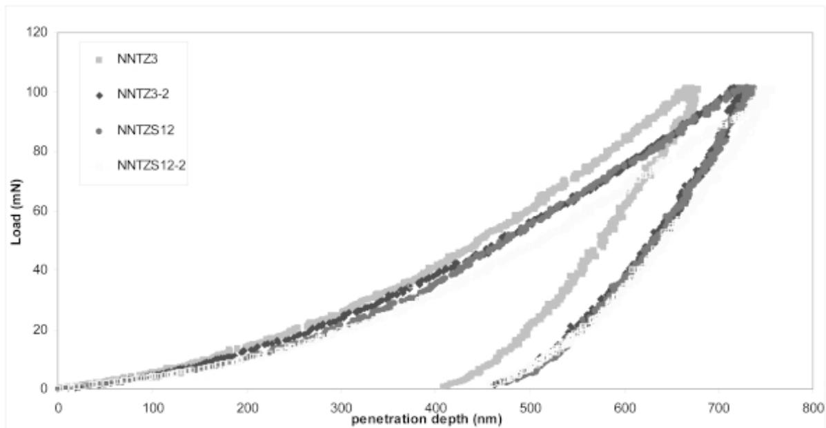
**Fig. 10.** Depth-Load curves recorded during dynamic microhardness test of UHP compacted investigated alloys B (NNTZ3) and C (NNTZ12).
