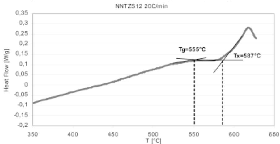
Fig. 7. DSC Analysis of the powder of alloy C milled for 60 hours.
