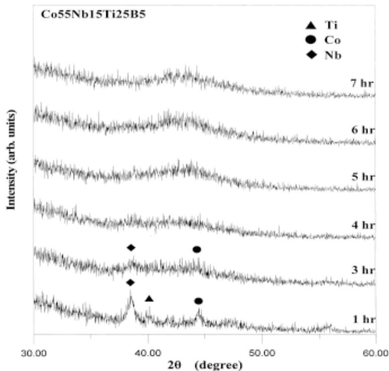
Fig. 1. XRD patterns of the milled  $\text{Co}_{55}\text{Nb}_{15}\text{Ti}_{25}\text{B}_5$  powder at different milling times.
