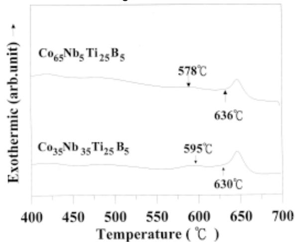
Fig. 2. DSC curves for the  $\text{Co}_{65}\text{Nb}_5\text{Ti}_{25}\text{B}_5$  and  $\text{Co}_{35}\text{Nb}_{35}\text{Ti}_{25}\text{B}_5$  alloys.
