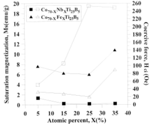
**Fig. 4.** Variations of saturation magnetization and intrinsic coercive force with Fe or Nb atomic percent for the  $\text{Co}_{70-X}\text{Fe}_X\text{Ti}_{25}\text{B}_5$  and  $\text{Co}_{70-X}\text{Nb}_X\text{Ti}_{25}\text{B}_5$  powders. Full symbols represent saturation magnetization and open symbols represent coercive force.
