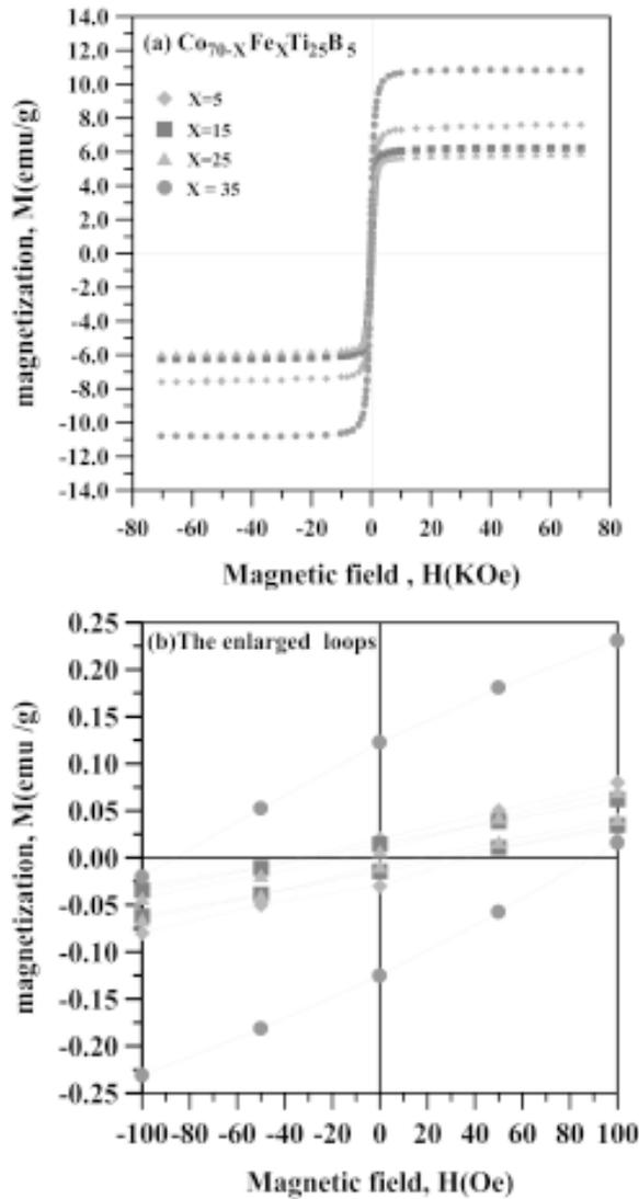
**Fig. 3.** (a) M-H loops of the milled  $\text{Co}_{70-X}\text{Fe}_X\text{Ti}_{25}\text{B}_5$  powders, and (b) the same M-H loops in an enlarged scale.
