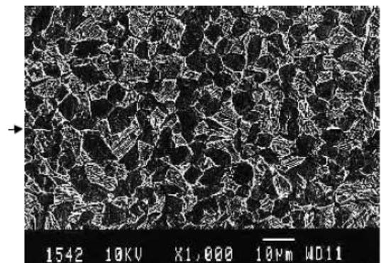
Fig. 2. Micrographs of the solid state joint for the VT6 alloy after pressure welding at  $900 \text{ }^\circ\text{C}$ .
