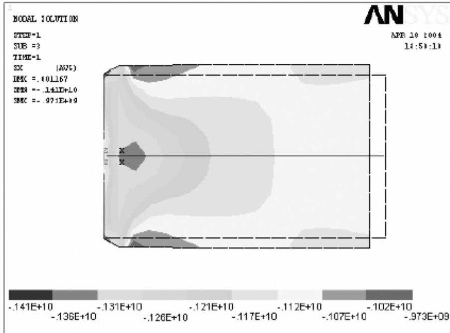
Fig. 5. Pattern normal effort with contact square of cross section.
