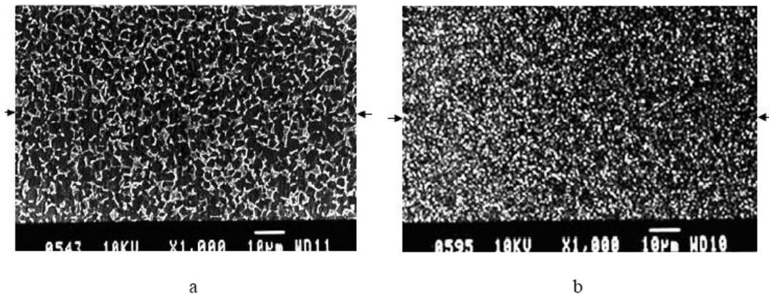
Fig. 3. Micrographs of the solid state joint for the VT6 alloy after pressure welding at 800 (a) and 700 °C (b).
