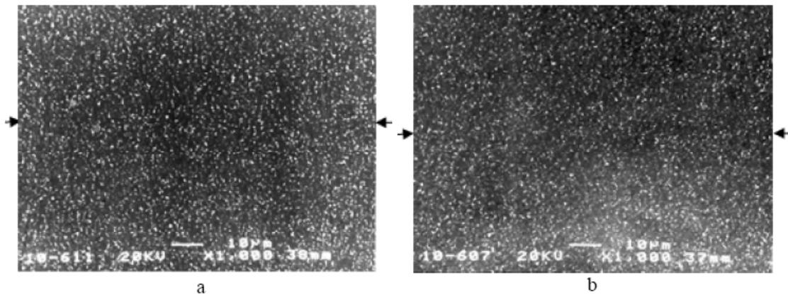
Fig. 9. Micrographs of the solid state joint for the VT6 alloy after pressure welding at 650 (a) and 600 °C (b) under conditions of low temperature superplasticity.
