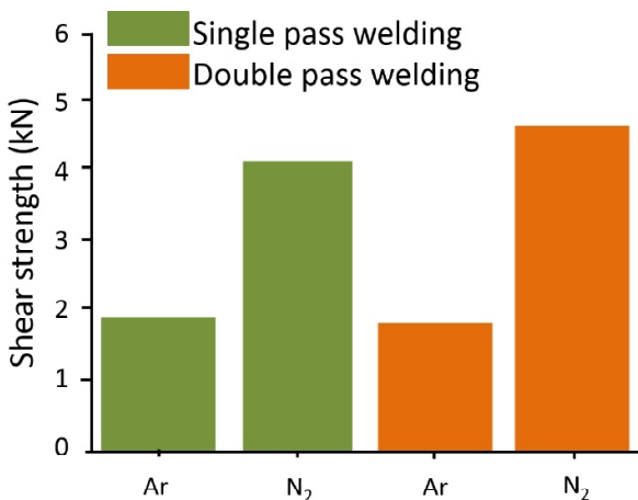
Fig. 7. Comparison between the effect of Ar and N 2 shielding gases on the shear strength of the laser welded lap joint of Zn-coated steel (DX54) and Al alloy (5754), using either single pass or double pass fibre laser (first pass welding parameters: 650 W, 100 mm/s, f.p.p. of 0 mm, second pass welding parameters: 200 W, 75 mm/s, f.p.p. of +2 mm), reprinted with permission from H.C. Chen, A. J. Pinkerton, L. Li, Z. Liu and A.T. Mistry // Mater. Des. 32 (2011) 495, (c) 2011 Elsevier.
